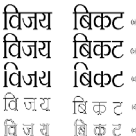
Fig. 6 Preprocessed images (a) Original, (b) Segmented Image, (c)Shirorekha Removed, (d) Thinned, (e) Image Edging.
