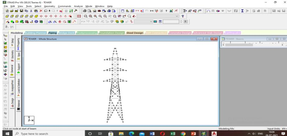
Figure 4 : Model developed in STAAD Pro
