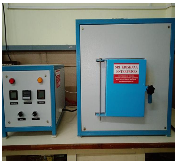
Fig. 1: Furnace used for melt quenching
