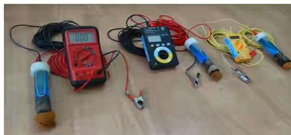
Fig: Equipment For Half Cell Potential Method
