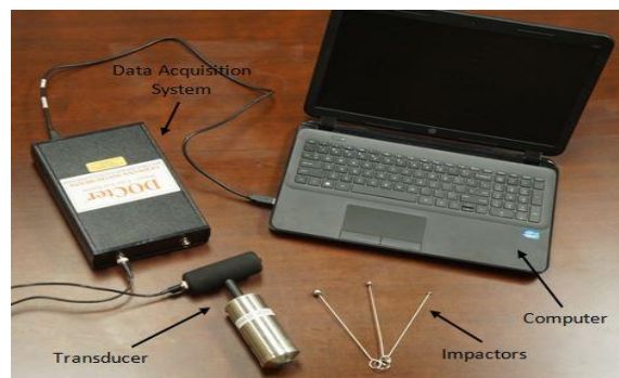
Fig: Equipment for Impact Echo Test
