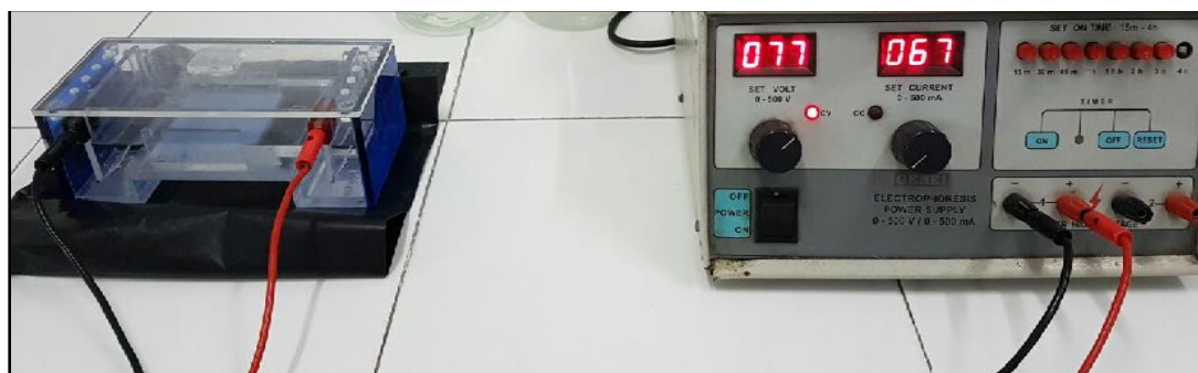
Fig.1.2. Gel Electrophoresis set up to quantify amplified DNA isolated from the sample collected.
