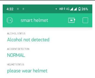
• The rider has consumed alcohol or not is detected and in case if he has consumedmeans vehicle will not turn on else it will turn on.
