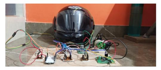
The above snapshot contains all the hardware parts such as Pressure sensor, Alcoholicsensor, Tilt sensor, Microcontroller, Dcmotor and Helmet
