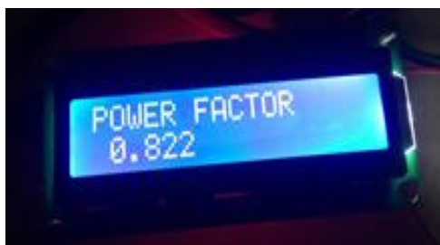
Fig 6.1.3 Power factor output with SEPIC converter
