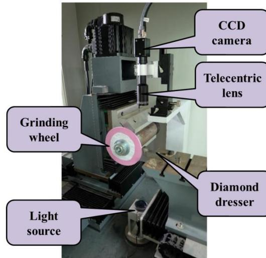
Figure 6: Self-developed profile grinding testbed.
