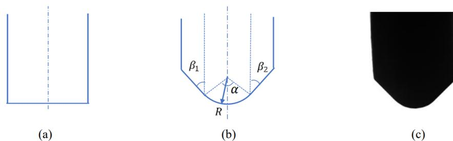
Figure 7: The nose shape of the wheel (a) original profile; (b) theoretic profile; (c) actual profile.
