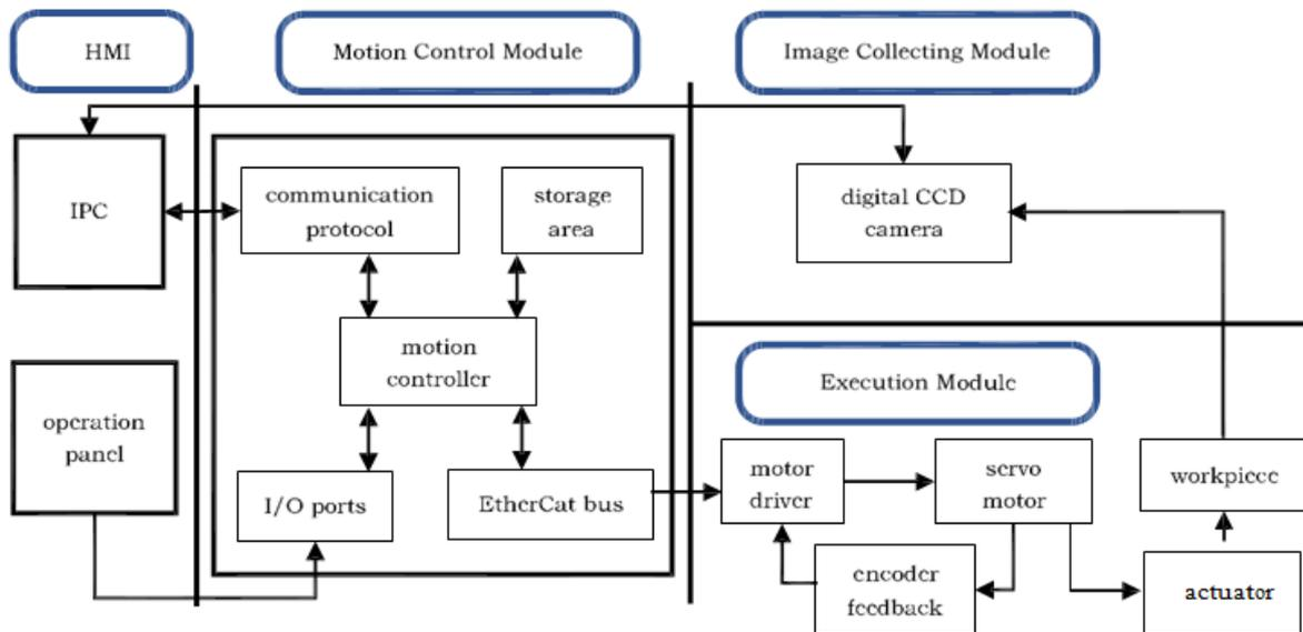
Figure 2: Hardware structure of open profile grinding CNC
