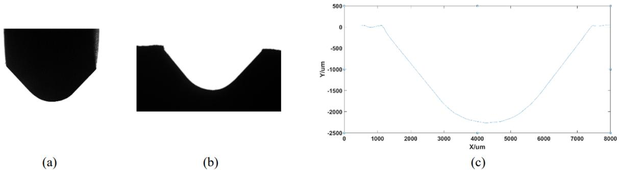
Figure 8: Profile measurement based on different methods (a) grinding wheel image; (b) profile copy image; (c) profile measured by optical profiler.
