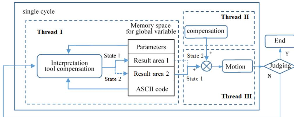
Figure 4: The process of multi-thread accessing memory space.
