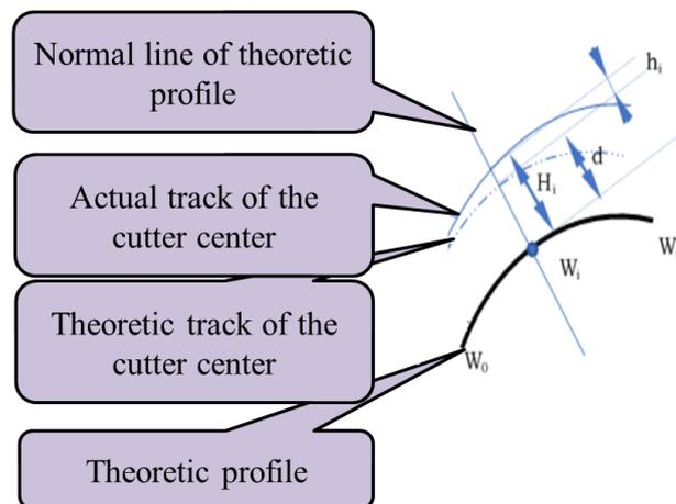
Figure 9: Quantification of actual machining trajectory errors.
