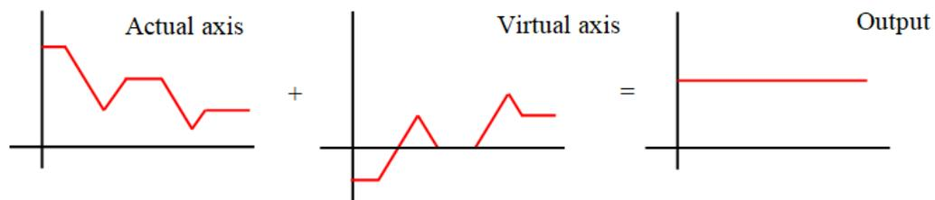
Figure 5: Virtual axis based compensation mechanism
