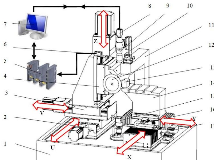
**Figure 1: Structure of profile grinding machine.**
