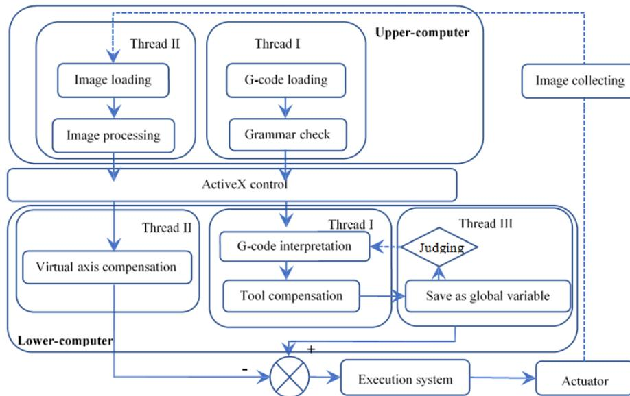
Figure 3: The structure of CNC system software.
