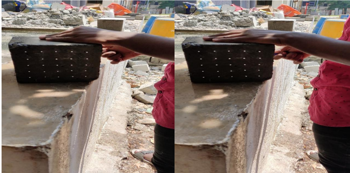
TRANSPARENT CONCRETE BY NATURAL LIGHT
