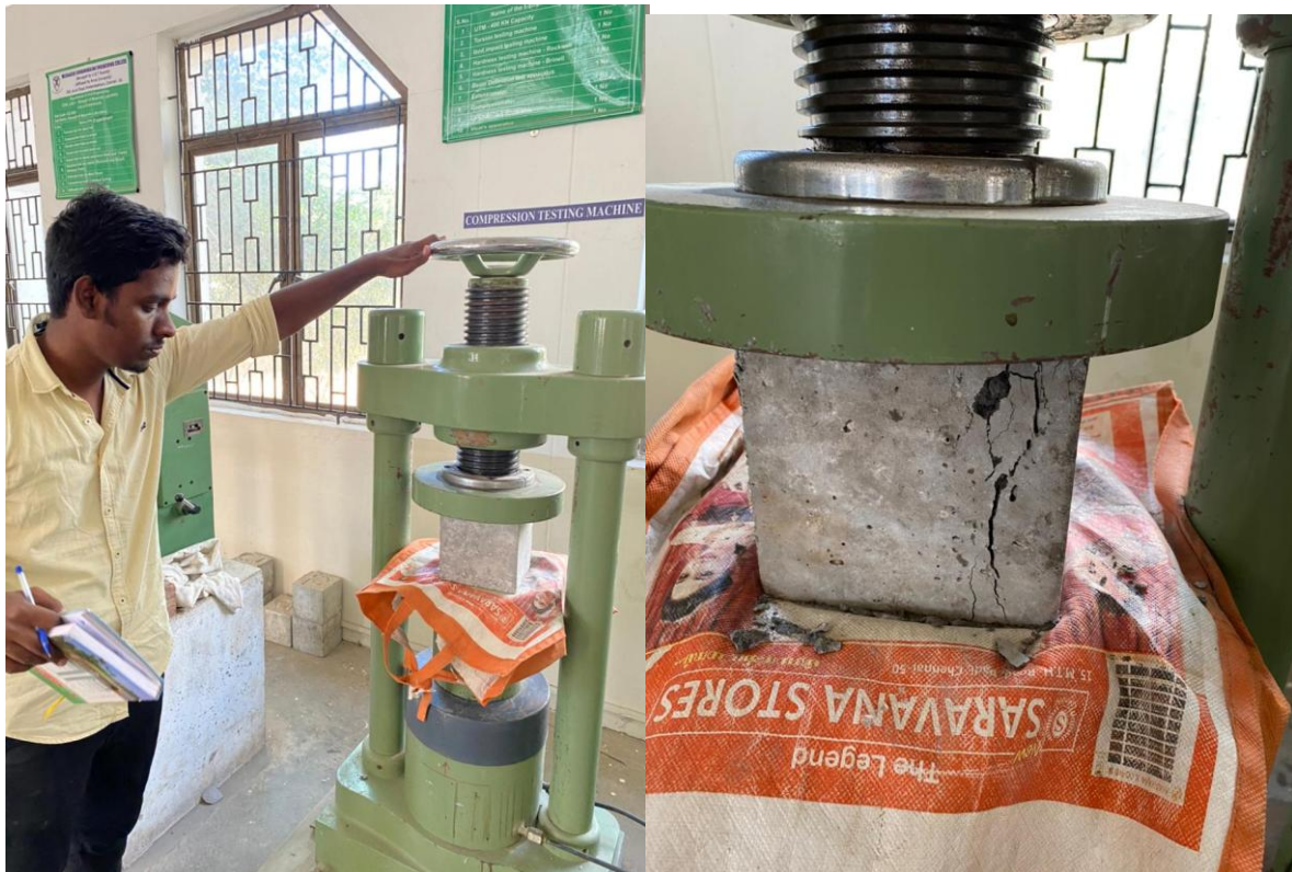
TRANSPARENT CONCRETE IN CTM MACHINE
