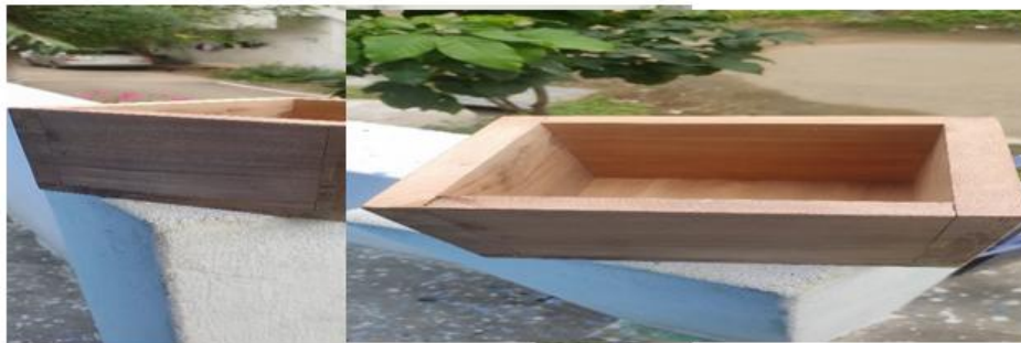
WOODEN CONCRETE MOULD
