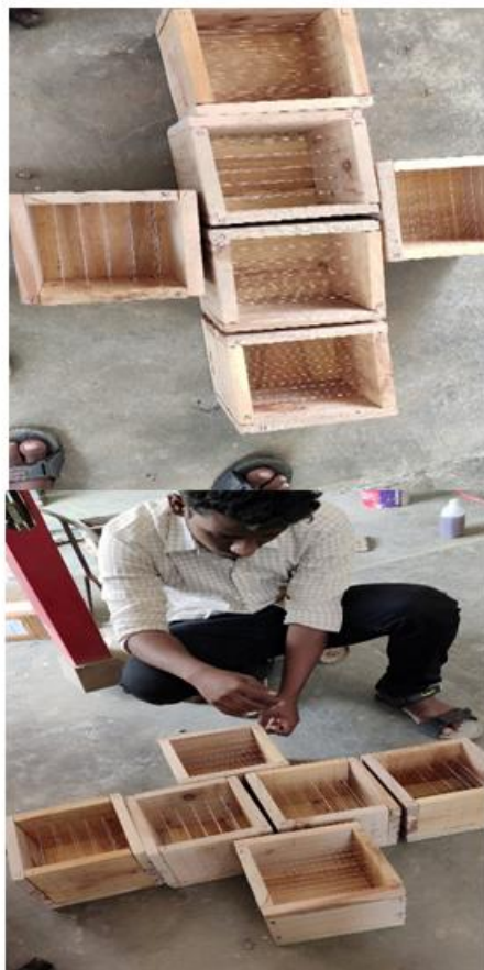
INSERTING OPTICAL FIBRE IN MOULD
