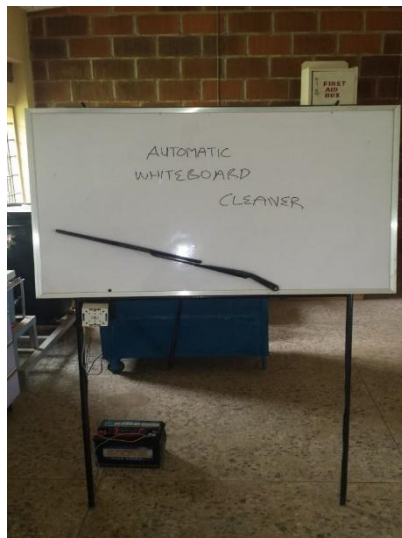
Figure 4: Automatic whiteboard cleaner hardware and its electrical connection
