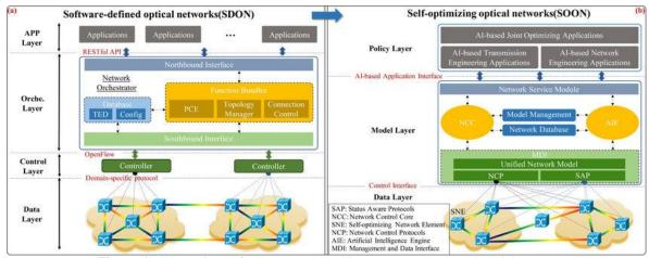
Figure 1. Comparison of two network architectures : a) SDON ; b) SOON [1].
