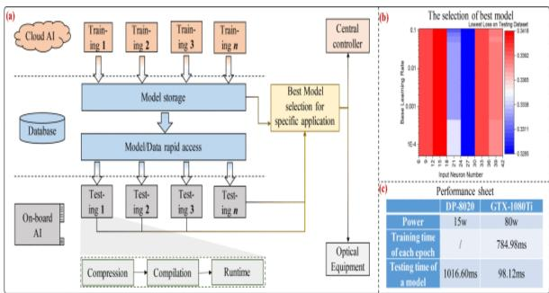
**Figure 4**.Cross layer optimization : a) Collaboration training and testing and of models ; b) the selection of best model ; C) the performance sheet of control-layer AI and on-board AI [1].
