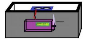
When the dustbins are about to get full, the level of garbage in the bin is detected by the ultrasonic sensors. These two sensors are set in both the dustbins to sense and send the details to the Arduino. If the bin is full, the message is sent to the municipal waste department with the location of dustbins using gsm module. The location is programmed in the Arduino code.
