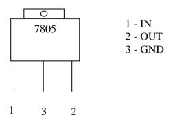
IN 7805 pin no.1 is input pin through which non-regulated signal is used. Pin no.3 is grounded and regulated output is taken from pin no.2.
