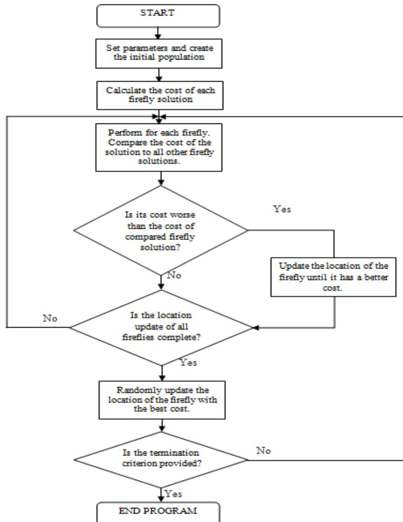
**Figure 2. Flowchart of firefly algorithm**
