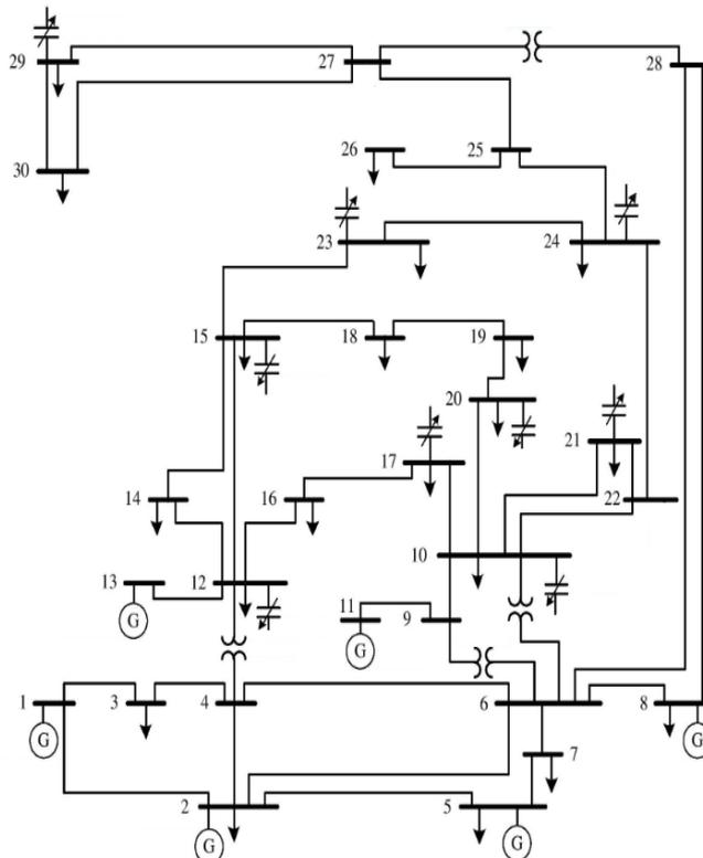
Figure 3. IEEE30-busbar test system [23]
