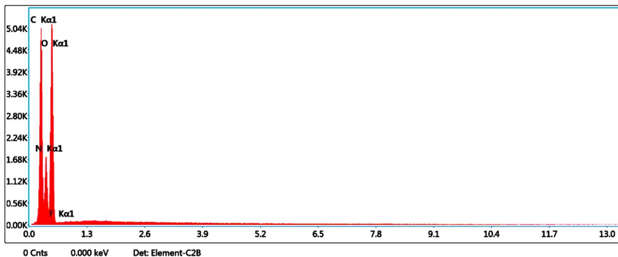
**Fig. 9: EDX spectrum for glycine hydrofluoride crystal**
