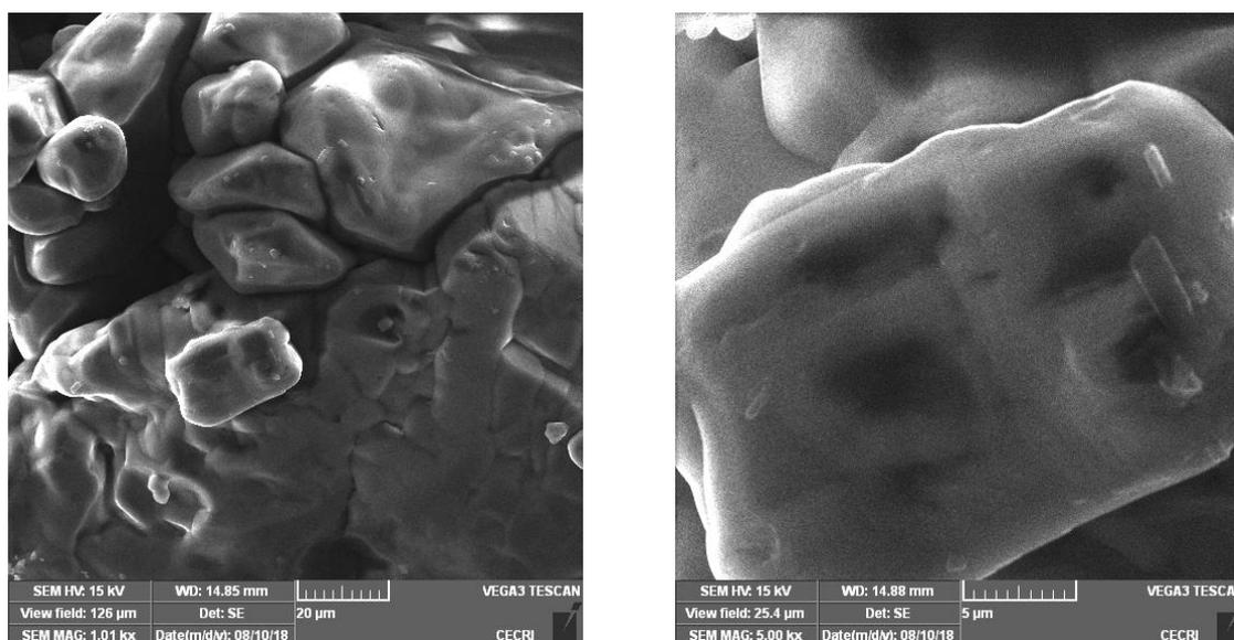
**Fig. 8: SEM photograph for glycine hydrofluoride crystal**
