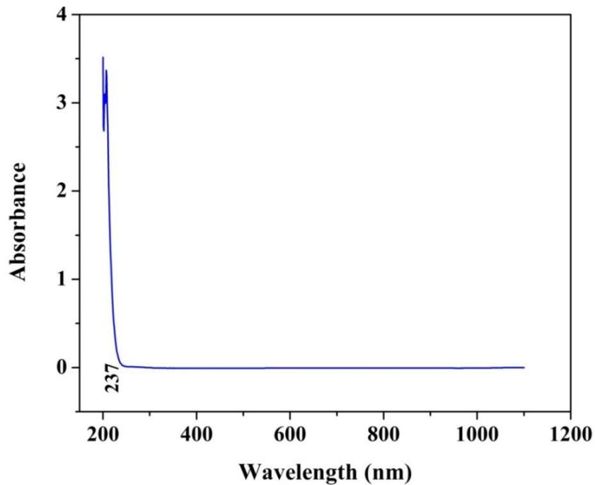
**Fig. 6: Absorbance spectrum for glycine hydrofluoride crystal**
