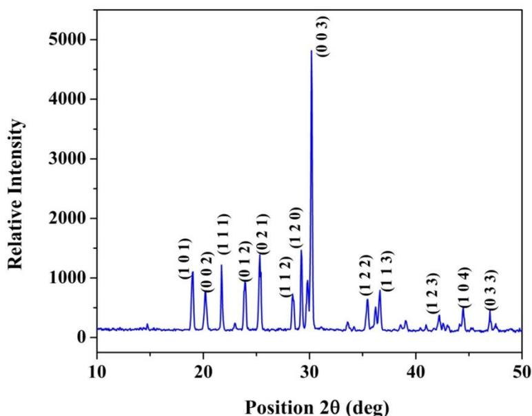
**Fig. 3: Diffraction patterns for glycine hydrofluoride crystal**
