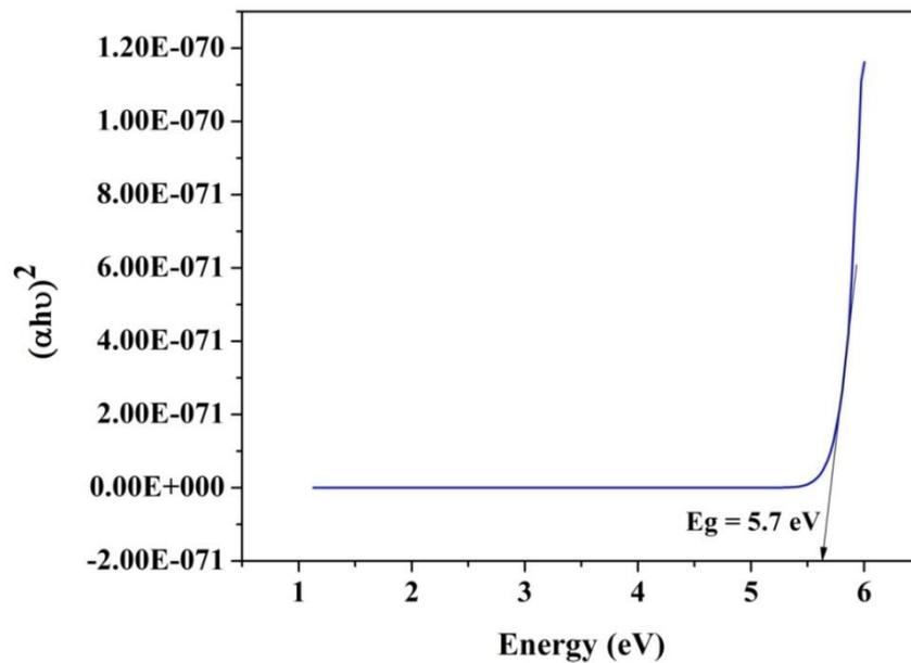
**Fig. 7: Optical band gap for glycine hydrofluoride crystal**
