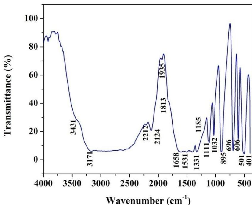
Fig. 4: FT-IR spectrum of glycine hydrofluoride crystal
