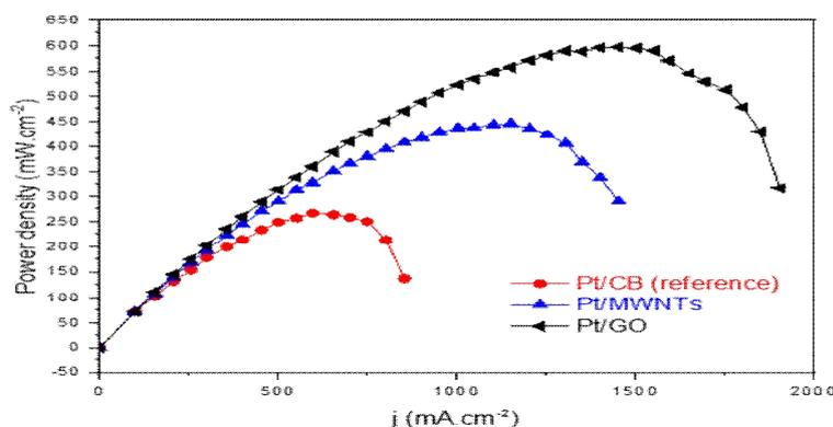
**Figure 5.** Polarization tests of fuel cell Pt/GO, Pt/MWNTs and Pt/CB (used as a reference).
