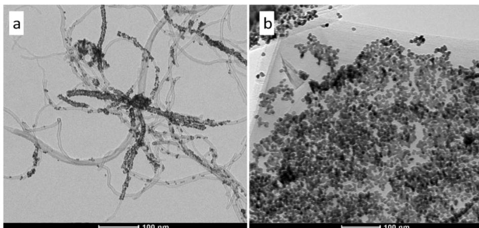
Figure 2. TEM micrographs of Pt/MWNTs (a) and Pt/GO (b) systems.
