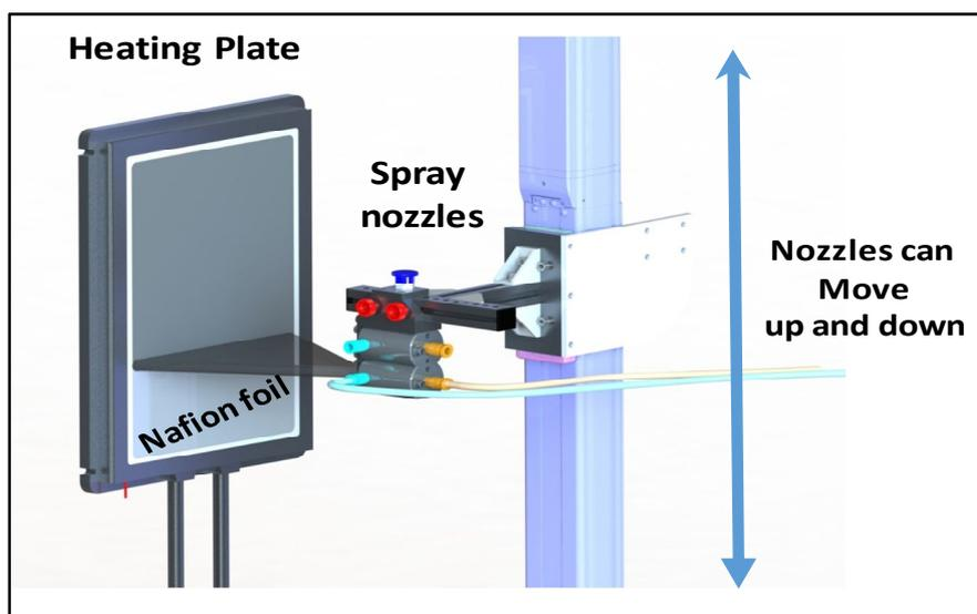
**Figure 1.** Schematic representation of the vertical spray prototype used for the deposition of Pt/Carbon nanomaterials. The nozzle was placed at a distance of 15 cm from the Nafion. The up and down speed rate was  $10 \text{ cm} \cdot \text{s}^{-1}$ .
