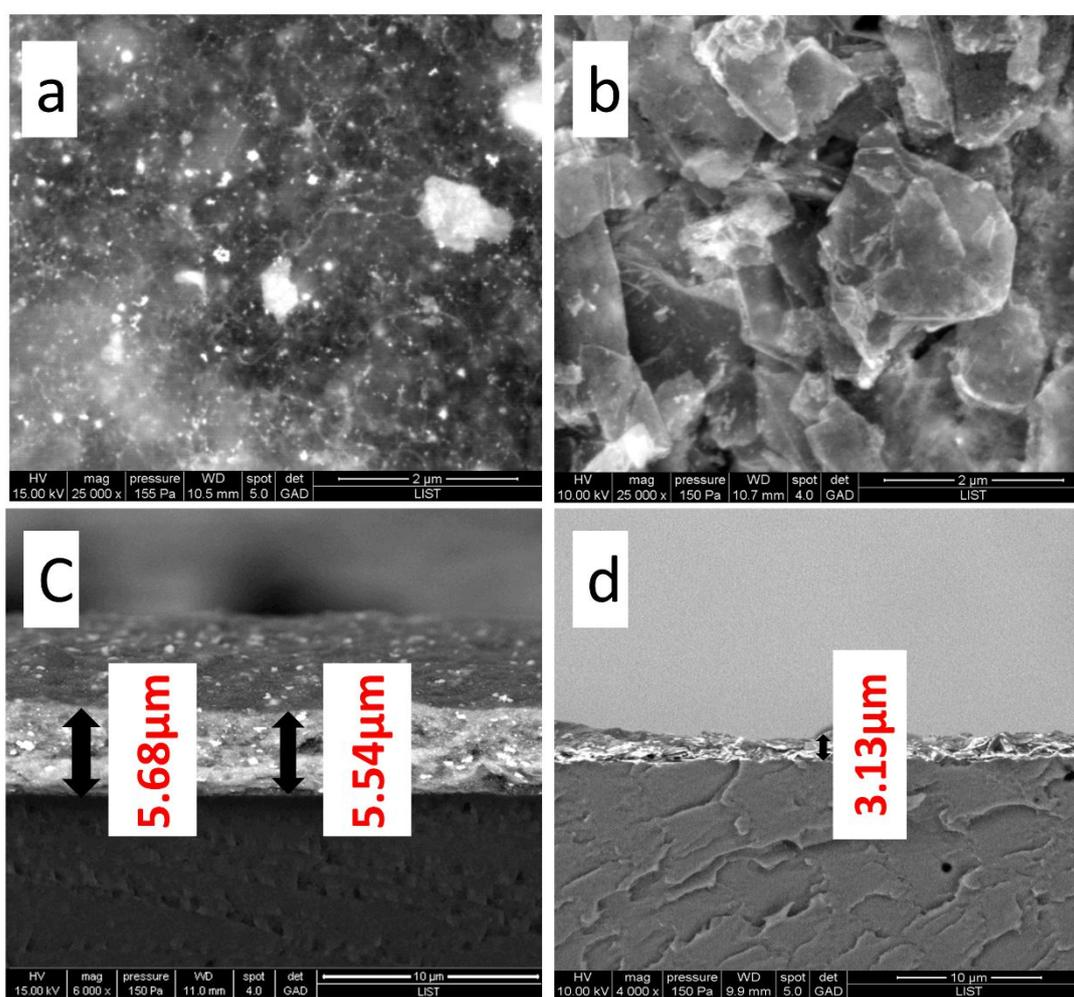
**Figure 3.** SEM micrograph top-views of (a) Pt/MWNTs and (b) Pt/GO electrodes and the cross-section of (c) Pt/MWNTs and (d) Pt/GO electrodes.
