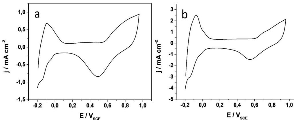
**Figure 4.** Voltammograms cycles (1800 cycles) of Pt/MWNTs (a), Pt/GO (b). Data were recorded in 0.5 M H<sub>2</sub>SO<sub>4</sub> at 25°C and a sweep rate of 50 mV.s<sup>-1</sup>.
