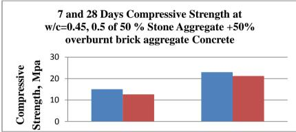
Graph 3: Compressive strength of 50% stone aggregate +50% Over-burnt brick aggregate concrete
