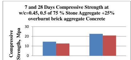
Graph 2: Compressive strength of 75% stone aggregate +25% Over-burnt brick aggregate concrete
