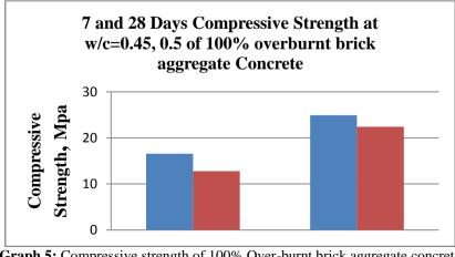
Graph 5: Compressive strength of 100% Over-burnt brick aggregate concrete
