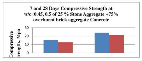
Graph 4: Compressive strength of 75% stone aggregate +25% Over-burnt brick aggregate concrete
