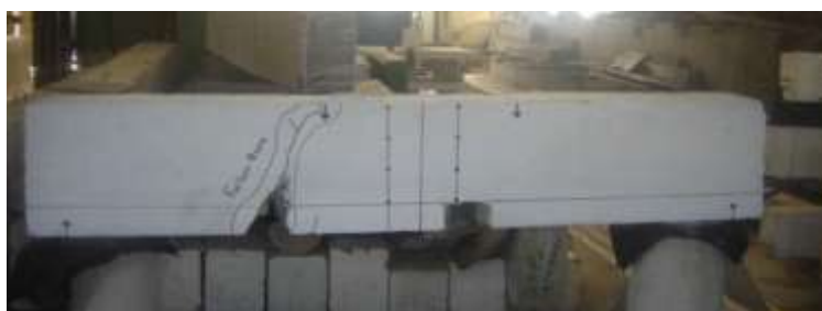
Figure 9 Failure Mode of Beam (B4)
