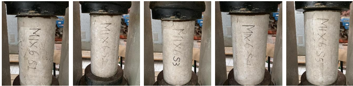
Figure 19. Failure mode of substitute 50% washed sea sand
