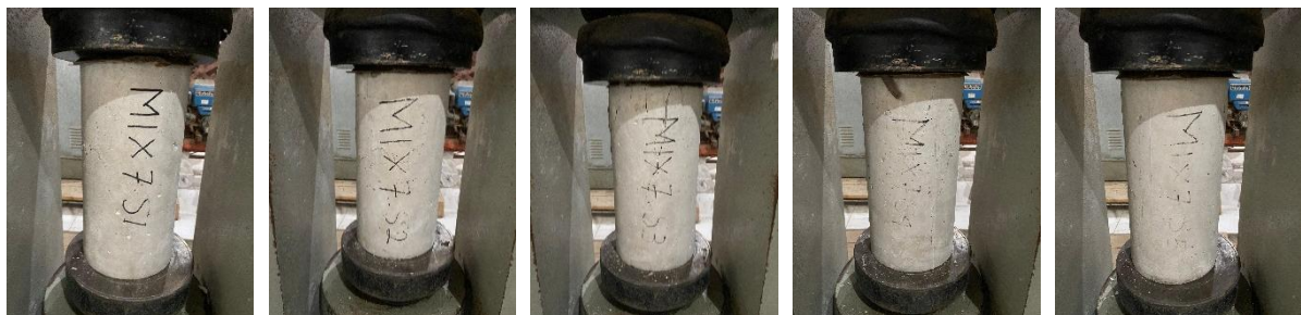
Figure 21. Failure mode of substitute 75% washed sea sand
