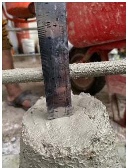
Figure 13. Slump test of concrete (75% of unwashed sea sand substitution)
