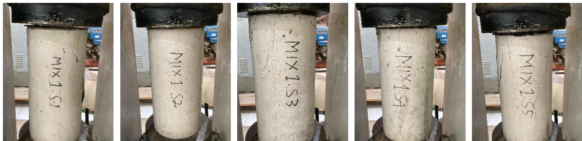
Figure 16: Failure mode of substitute 25% unwashed sea sand
