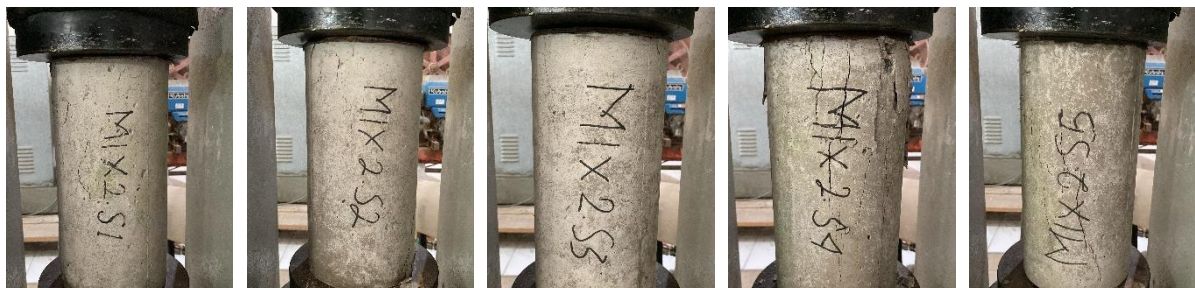
Figure 18. Failure mode of substitute 50% unwashed sea sand
