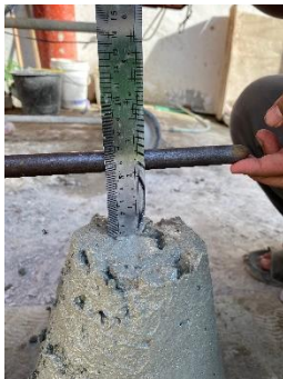
Figure 11. Slump test of concrete (50% of unwashed sea sand substitution)
