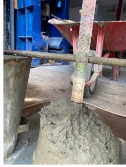
Figure 8. Slump test of normal concrete, none of sea sand
