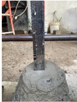
Figure 9. Slump test of concrete (25% of unwashed sea sand substitution)
