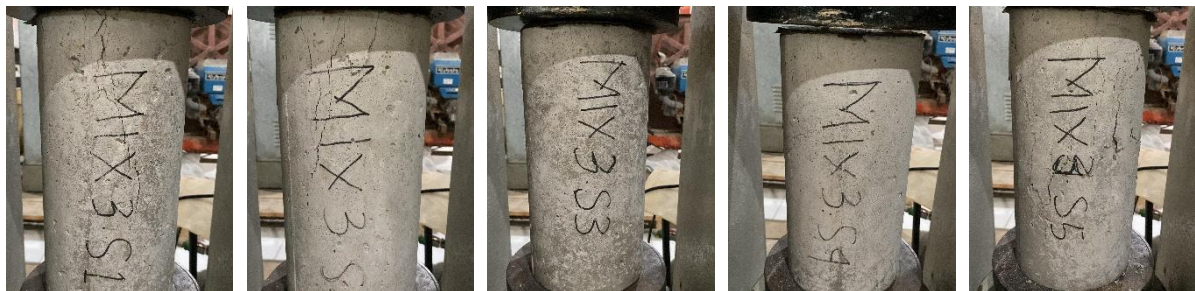
Figure 20: Failure mode of substitute 75% unwashed sea sand
