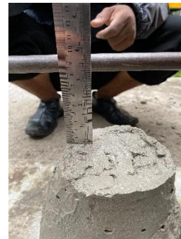
Figure 12. Slump test of concrete (50% of washed sea sand substitution)
