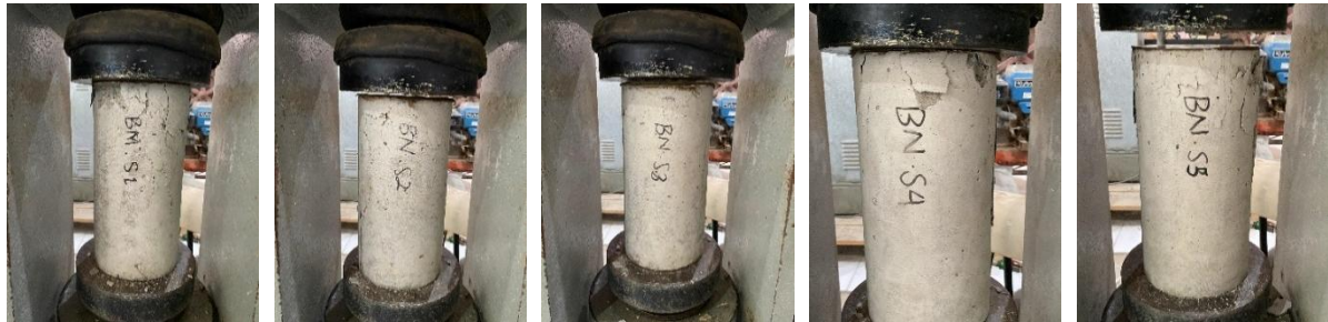
Figure 15. Failure mode of normal concrete
