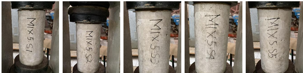
Figure 17. Failure mode of substitute 25% washed sea sand
