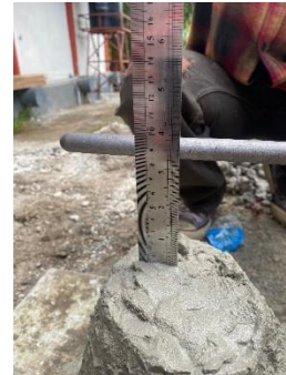
Figure 10. Slump test of concrete (25% of washed sea sand substitution)
