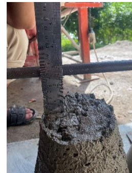
Figure 14. Slump test of concrete (75% of washed sea sand substitution)
