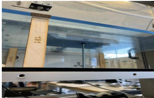
Figure 22 Flat glass plate for Setting ground clearance inside the wind tunnel
