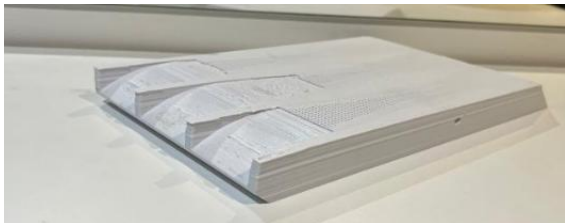
Figure 14: Failed Printed Model for Wind Tunnel Tests (isometric bottom view)
