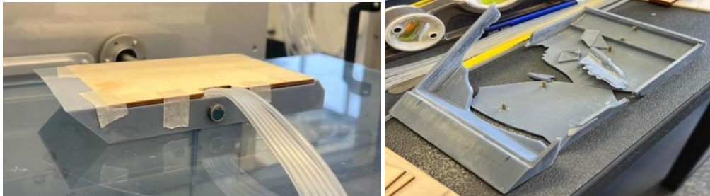
Figure 20 :Model Inside the wind tunnel (isometric view) figure 21.Model shown in a broken state after testing
