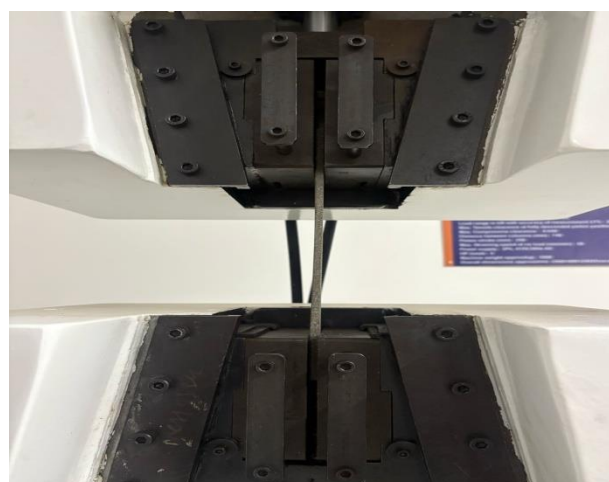
Fig 1.5.3: (universal testing machine for tensile)
