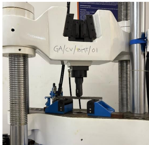
Fig 1.5.7:(universal machine for bending)
