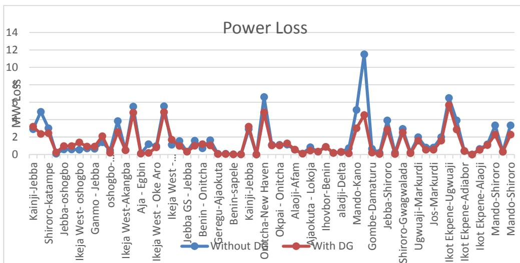
Figure 3.6: Line loss of the network after the DG has been connected.
