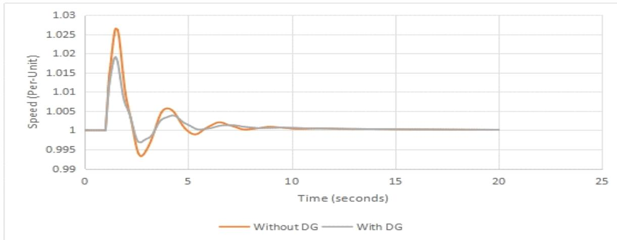
Figure 3.7: A plot of the speed against time with the connection of the Distributed generator.
