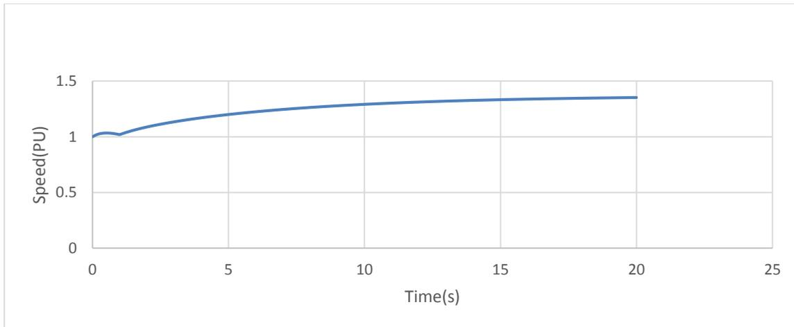
Figure 3.4: A plot of the speed against time without integrating to the transmission network.
