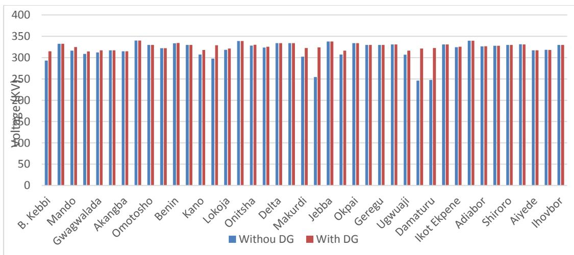
Figure 3.5: Showing the Bus Voltage of the Nigeria grid after the Distributed generators was connected.
