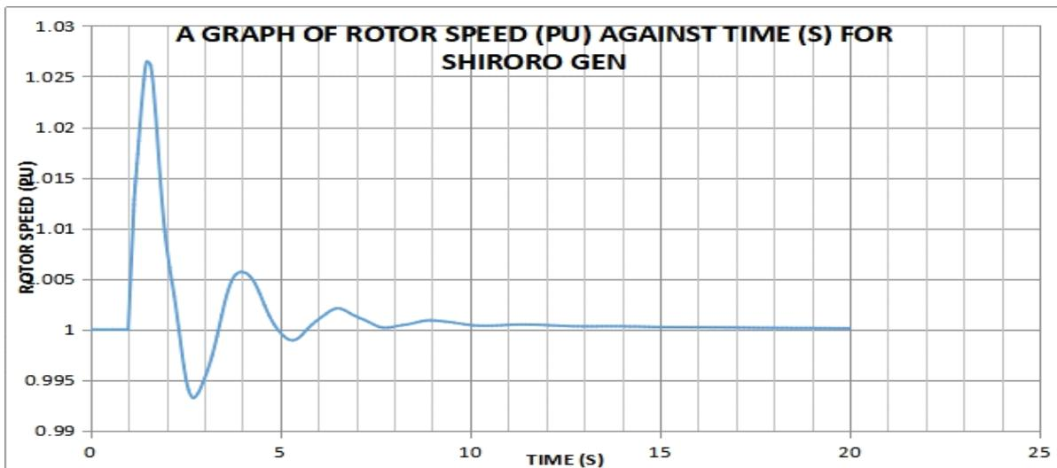
Figure 3.3: A plot of the speed against time without the connection of the DGs.
