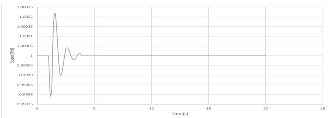
Figure 3.8: Plot of time against rotor speed after the integration to the transmission network.
