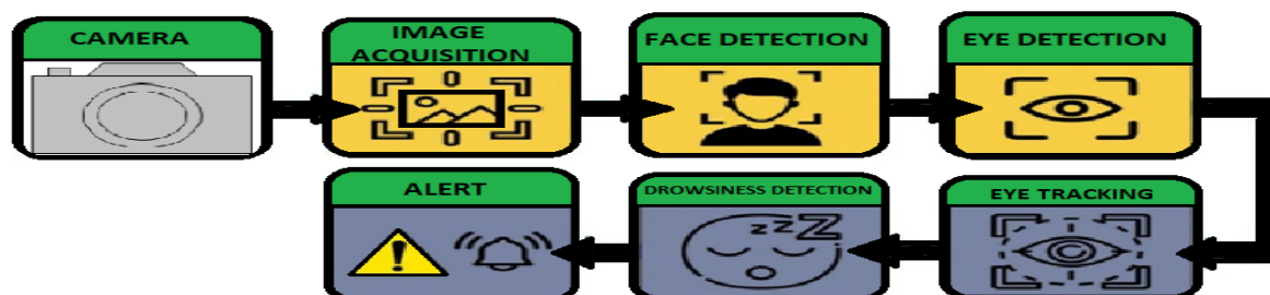
Fig. 4 Eye-blinking observation procedure
