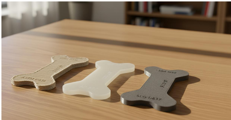
Figure 2: FDM, SLA, and SLS dog-bone tensile specimen post-printing.
