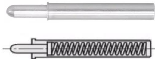
Figure13: The spring pin: physical object and internal structural diagram
