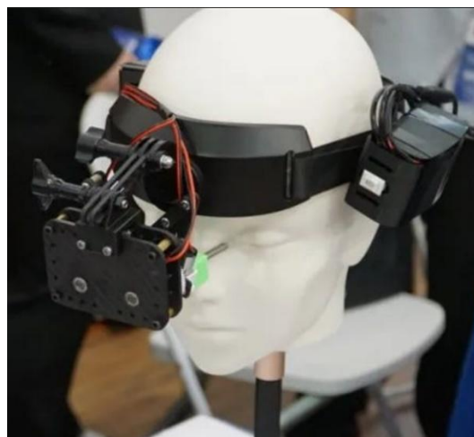
Figure16: The fabricated eye massager prototype
