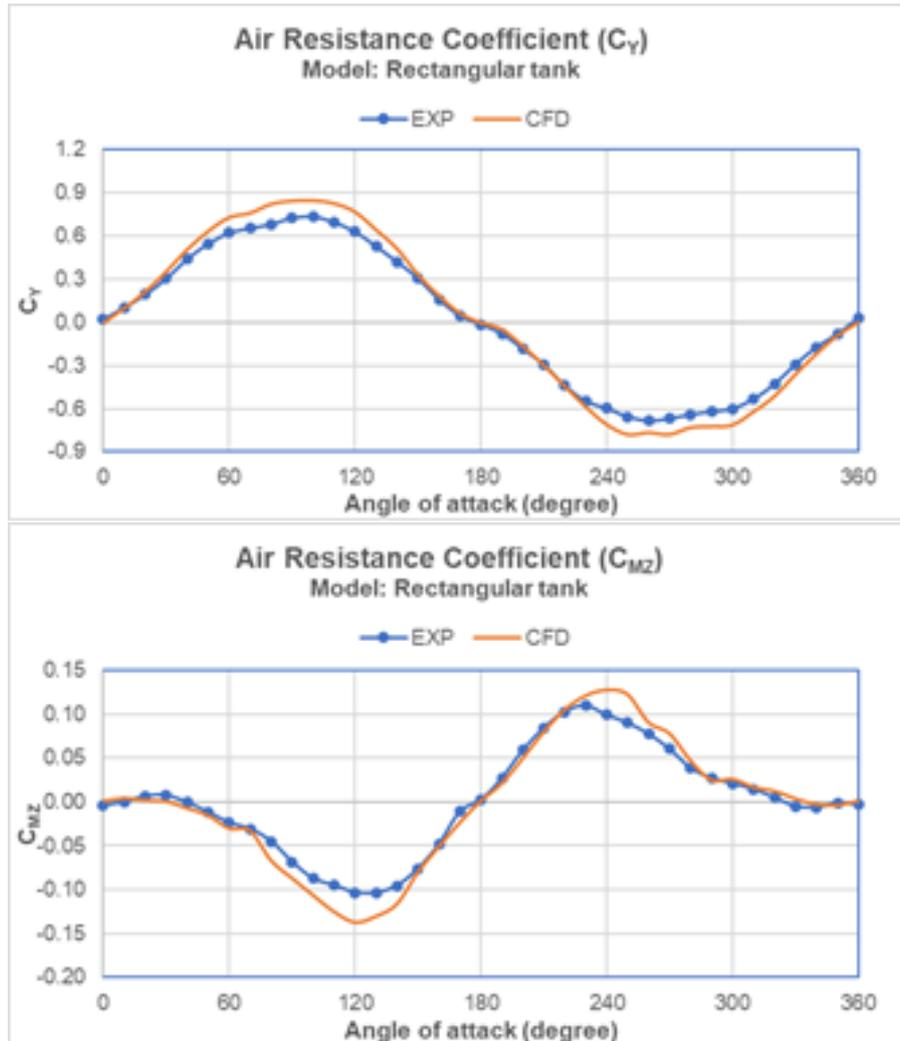
Figure 4: Air resistance coefficient – rectangular tank
