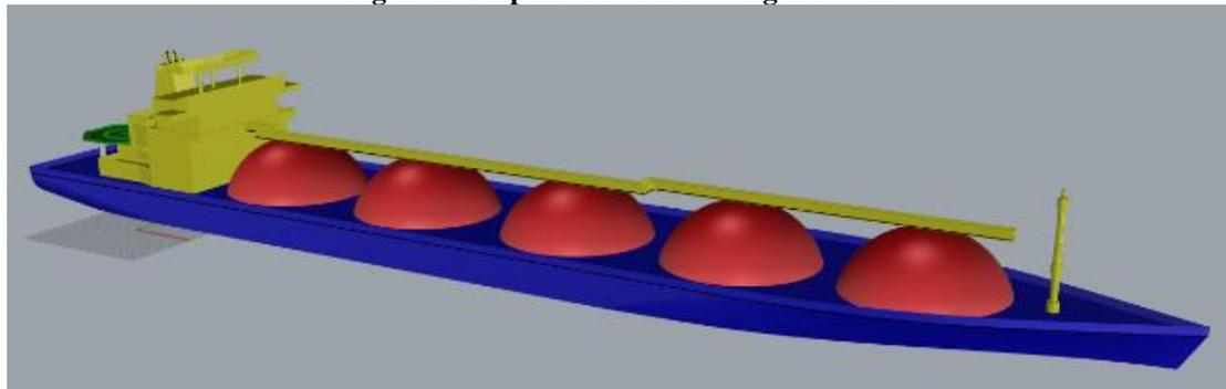
**Figure 2: Ship model with sphere tank**
