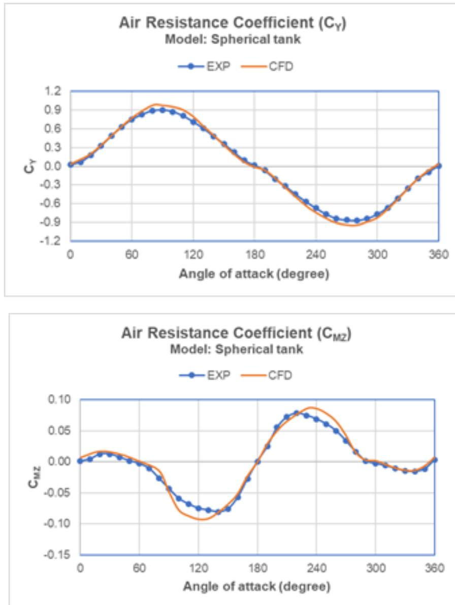
Figure 5: Air resistance coefficient – spherical tank
