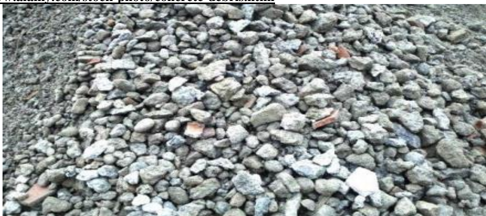
Figure 1.4 Recycled Concrete Aggregate
