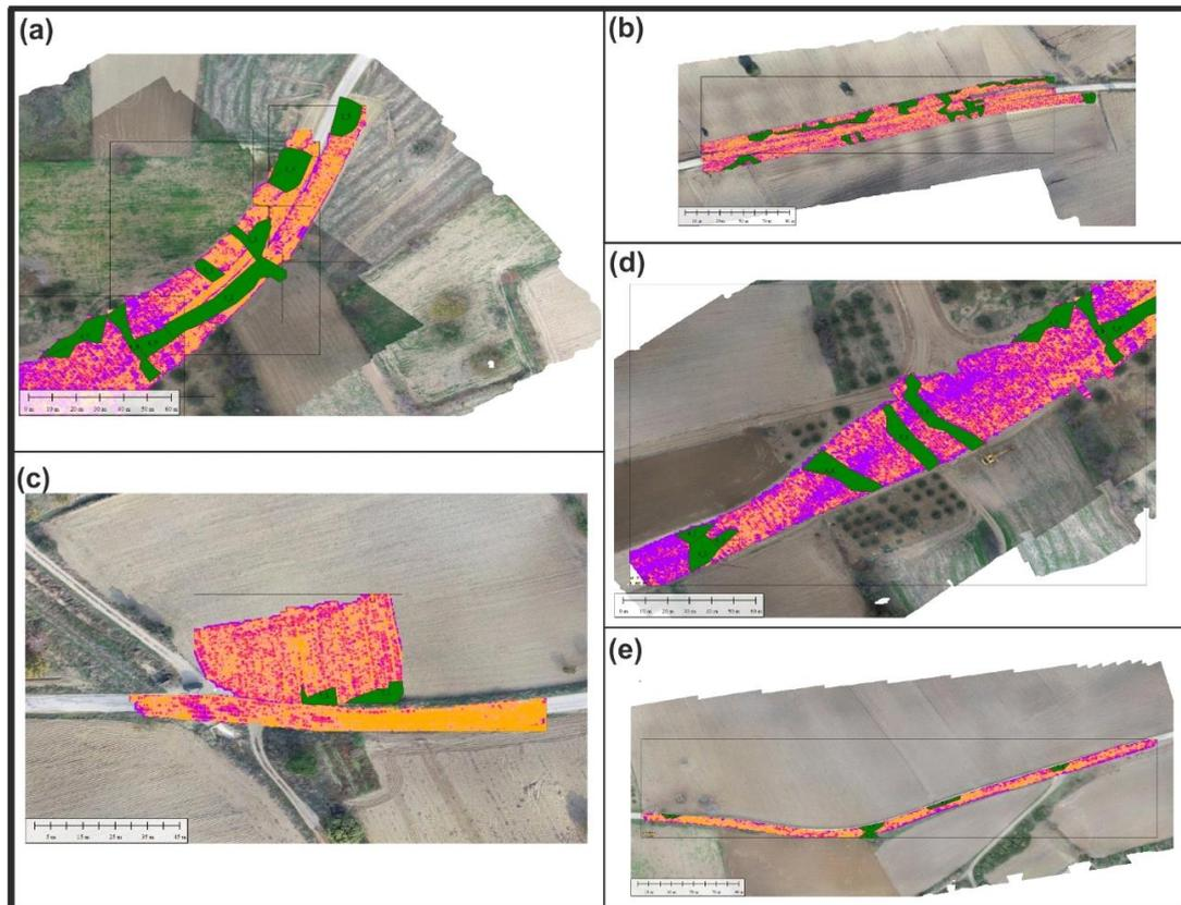
**Figure 9: Representation of GPR data and findings on the drone image generated for all regions (dark green areas correspond to anomalies).**
