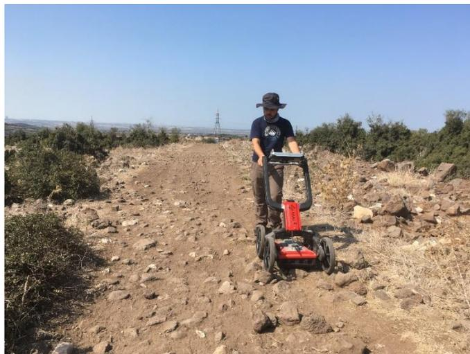
**Figure 2: GPR measurement applied in the study area.**
