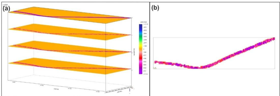
**Figure 8: In Region-5, (a) depth slices prepared for the measurement performed (b) selected optimal depth section (dark areas correspond to the anomaly)**
