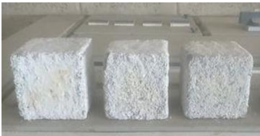
Figure: 1 Acid attacked specimen [14]
