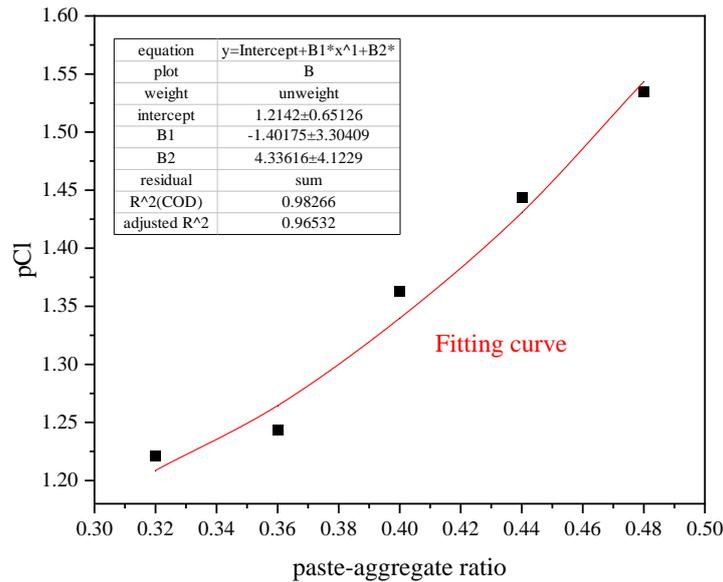
**Fig.8 Fitting curve of paste-aggregate ratio and diffusion coefficient**
