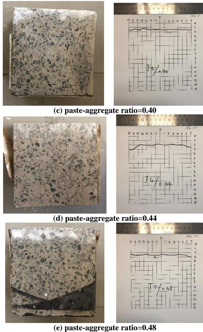
Fig.6. Curves of color development and erosion depth of specimen
