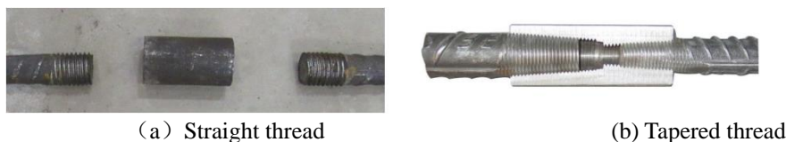
Figure 1.1 Threaded sleeve mechanical joint
