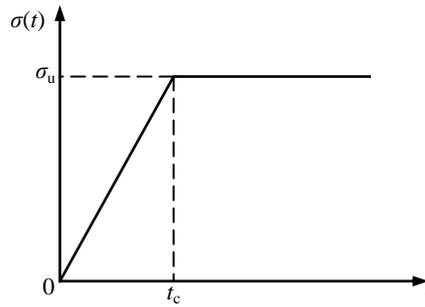
Fig.2  $\sigma(t)$ - $t$  curve under ramp loading
