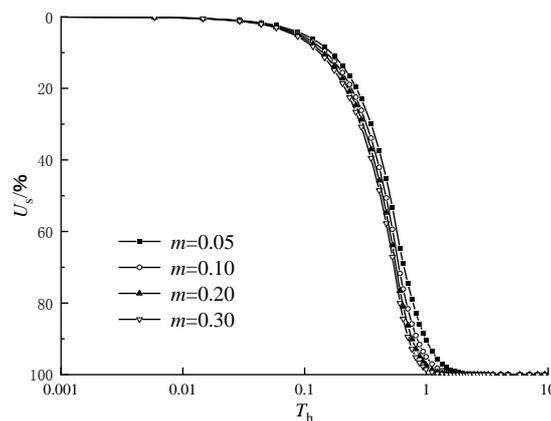
**Fig.7 Influence of replacement ratio of CCSG column with short core on consolidation rate**
