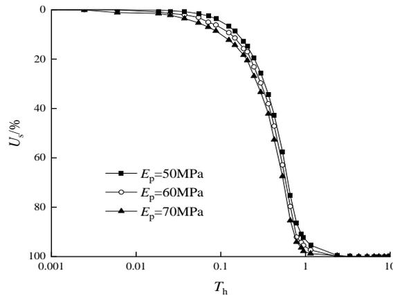
**Fig. 8 Influence of constrained modulus of stone shell ( column ) on consolidation rate**
