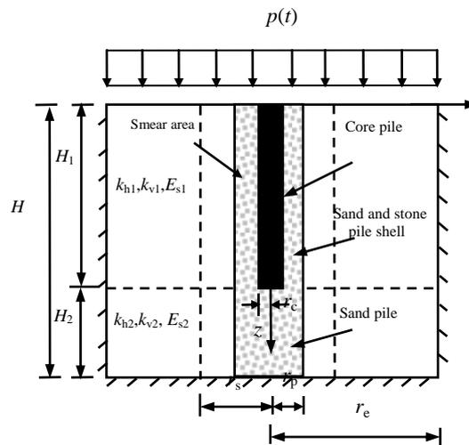
Fig.1 Axisymmetric consolidation model
