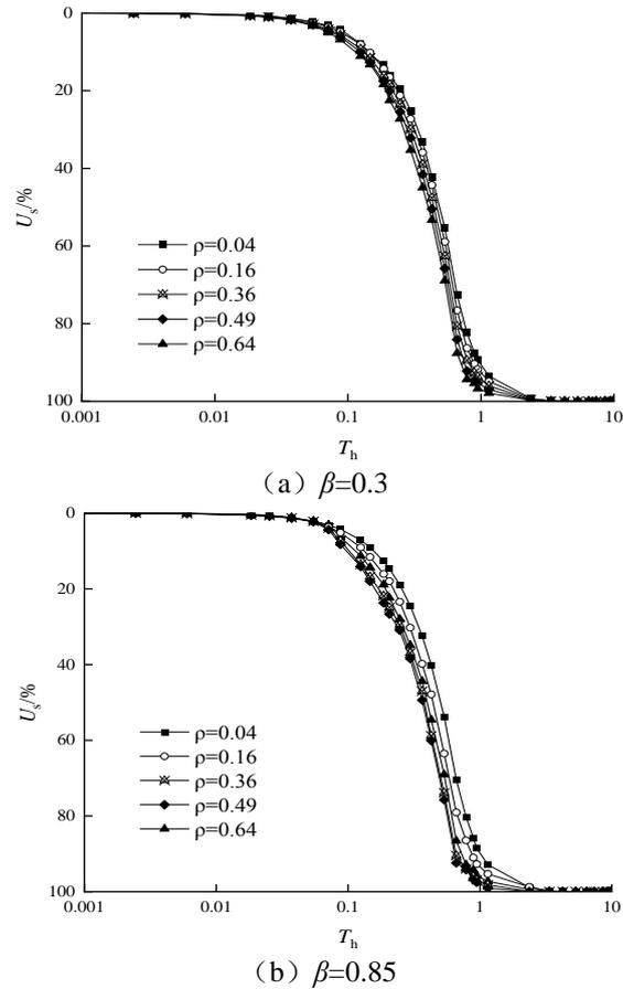
**Fig.5 Influence of area core ratio on consolidation rate**
