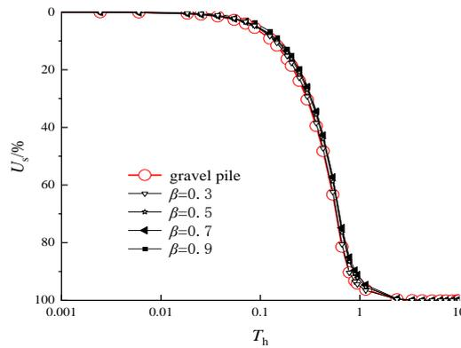
Fig. 4 Influence of core- column length ratio on consolidation rate
