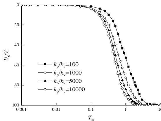
**Fig.9 Influence of permeability coefficient of stone shell (column) on consolidation rate**
