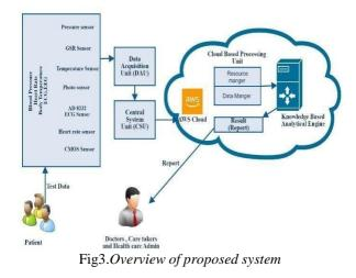
A) DAU-Used to collect physiologic data and send it to the Central System Unit for processing and verification of the data. PIN - Personal Identification Number codes are created for operator authentication purposes, together with identity cards. The DAU's Bluetooth module offers a wireless interface between the operator and the CSU.
