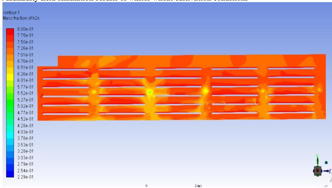
Figure 4.12 Relative humidity distribution cloud diagram on the vertical plane where the width is 1/2
