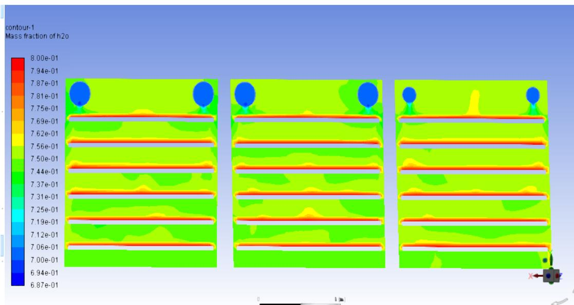
The relative humidity cloud diagram of the yz plane where the three groups of measuring points are located
