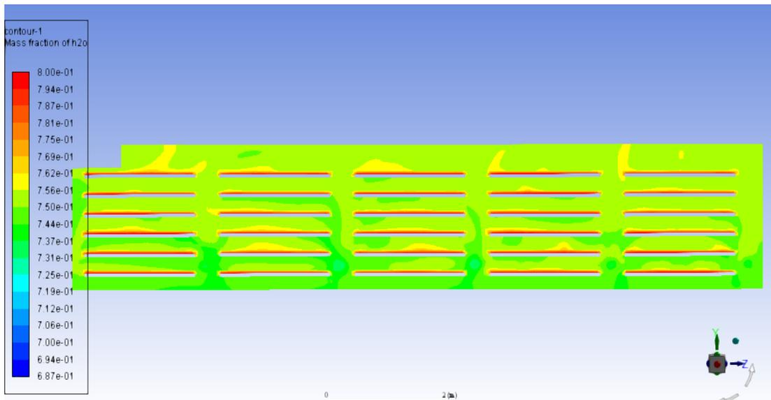
Figure 4.8 Relative humidity distribution cloud diagram on the vertical plane where the width is 1/2
