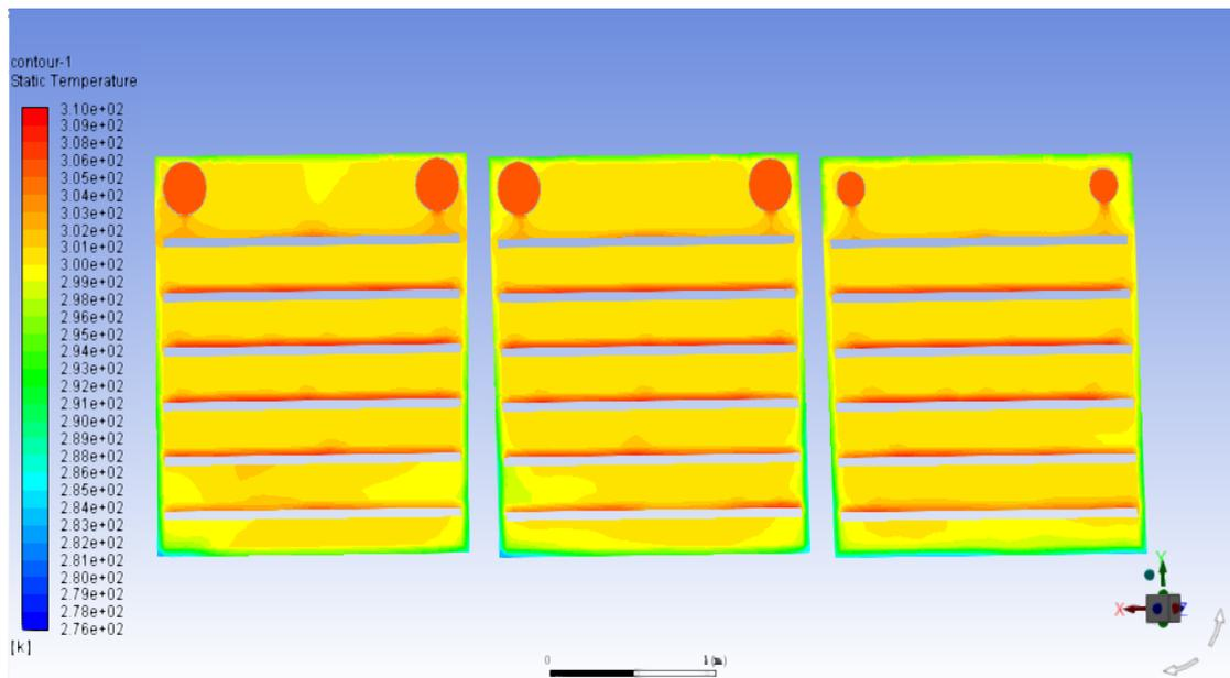
The temperature cloud diagram of the yz plane where the three groups of measuring points are located
