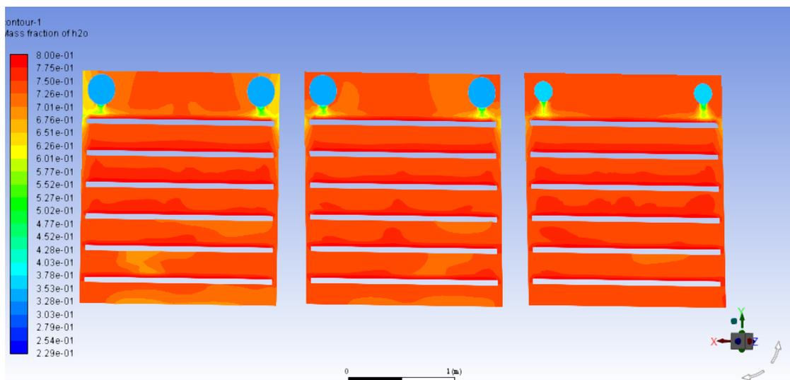
The relative humidity cloud diagram of the yz plane where the three groups of measuring points are located
