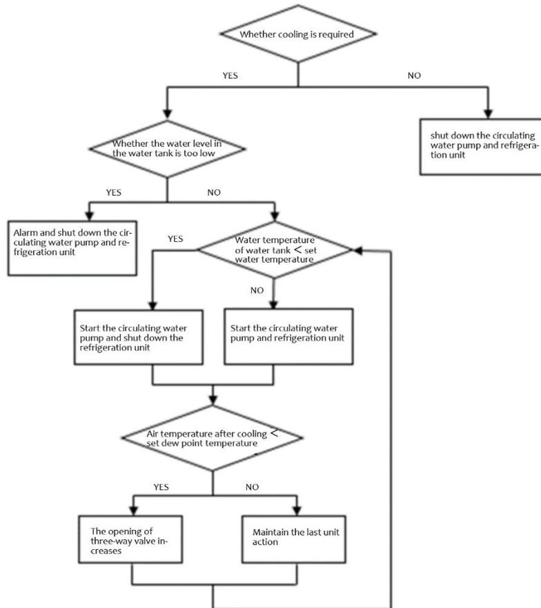
Figure 2.2 Logic diagram of cooling operation of air source heat pump unit
