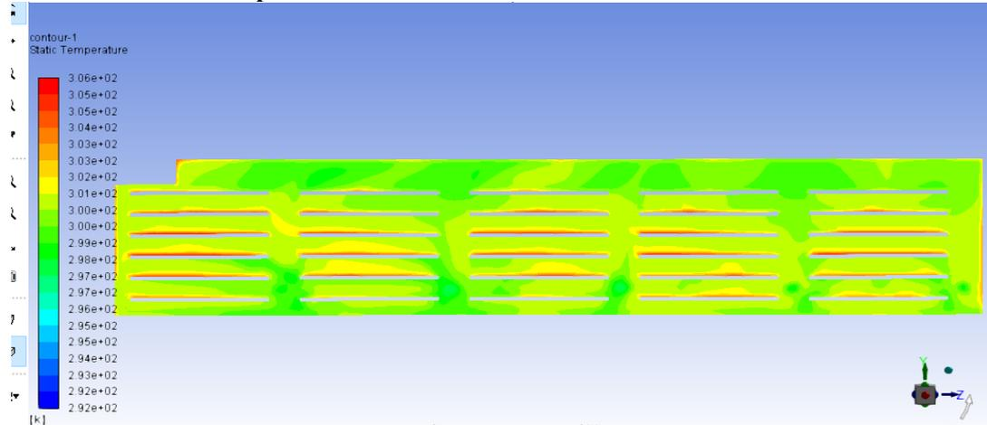
Figure 4.6 Cloud diagram of temperature distribution on the vertical plane of 1/2 width
