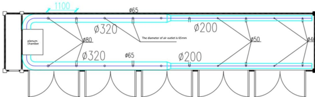
Figure 4.2 Floor plan of the air supply system in the box
