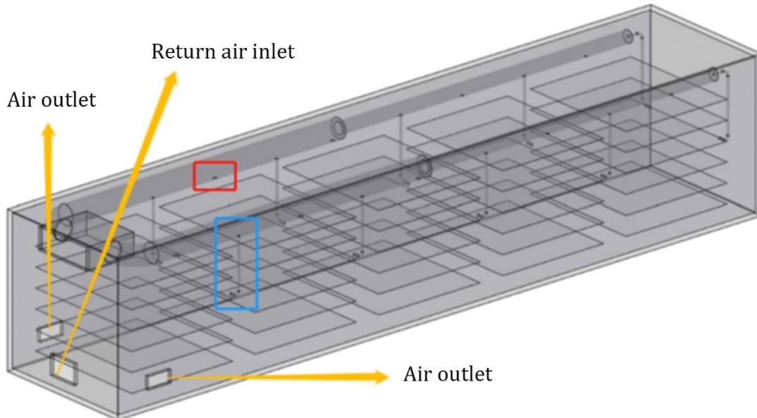
Figure 3.3 Three-dimensional model diagram of the incubator tuyere layout
