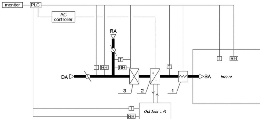
1 Electric heating 2 Surface heat exchanger 3 Mixing unit
