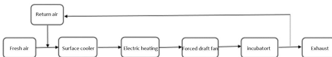
Figure 2.3 Flow chart of air treatment
