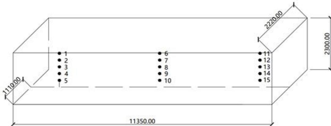
Figure 4.1 The observation surface and measuring point layout of the green feed cultivation container
