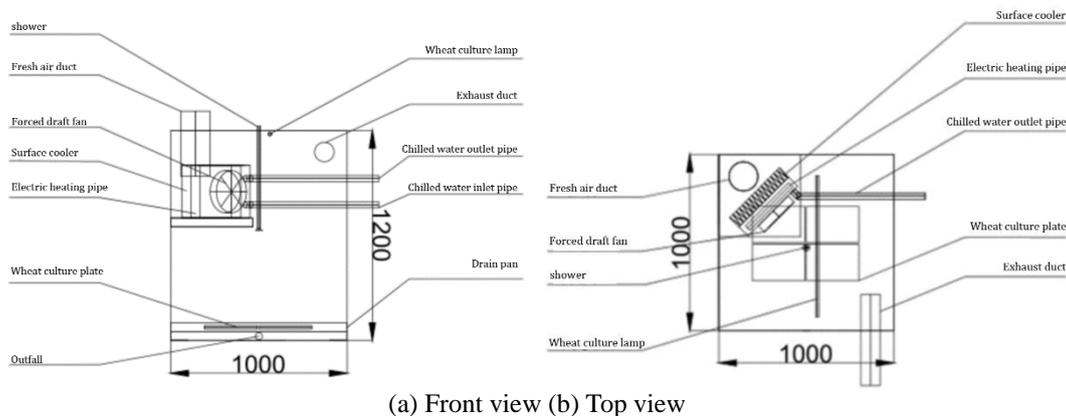
Figure 2.1 Schematic diagram of the structure of the wheat incubator
