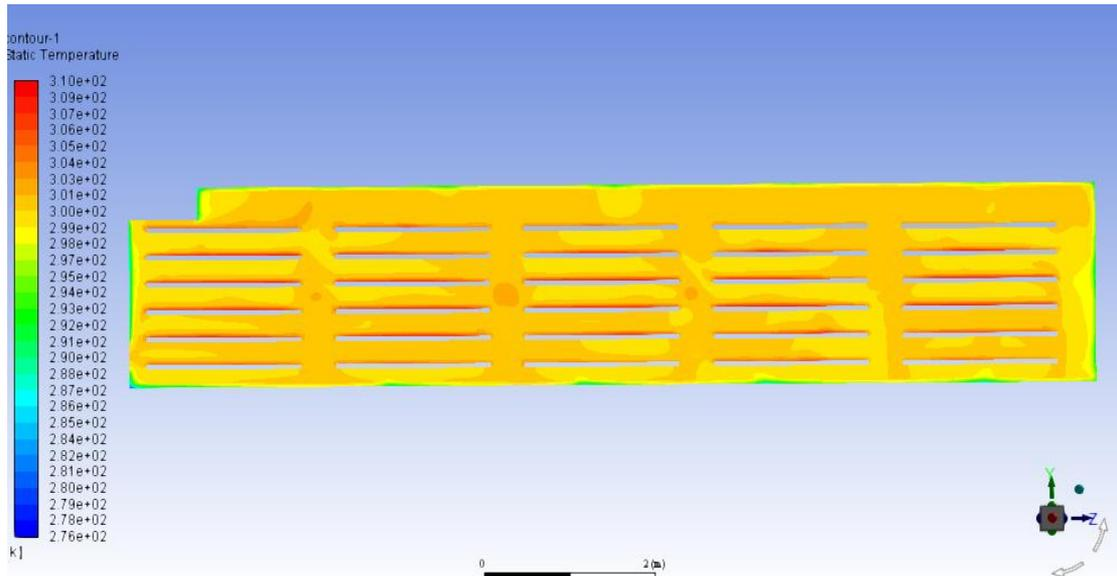
Figure 4.10 Cloud diagram of temperature distribution on the vertical plane of 1/2 width
