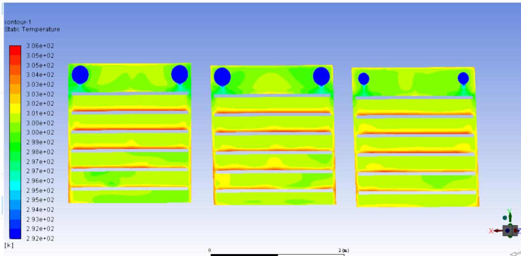
Figure 4.7 The temperature cloud diagram of the yz plane where the three groups of measuring points are located
