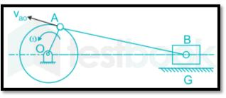
Figure 1: Sketch of slider crank
