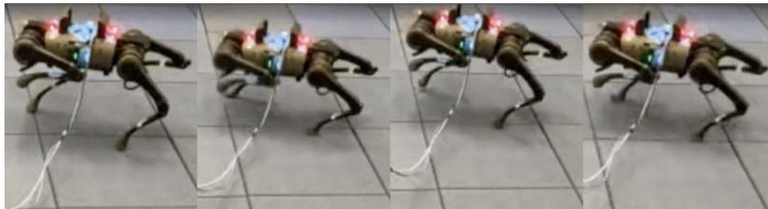
Figure 4.1: We evaluate our algorithm in quadrupedal locomotion tasks: catwalk and two-leg balance. The narrow feet placement and standing with two legs lead to falling easily during the learning process. Our algorithm overcomes these challenges—outperforming prior methods in terms of safety violations and learning efficiency both in simulation and the real world.
