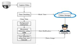
Fig1.Architecture of proposed system
