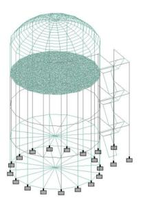
Whole Structure View of Combined Structure of Elevated Level Service Reservoir and Ground Level Service Reservoir.
