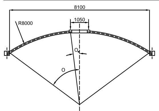
**Provide 8 Tor** @ **200 mm C/C Radially at top and 8 Tor** @ **200 mm C/C Circumferentially at top** Design of Top Slab (100 mm Thick)
