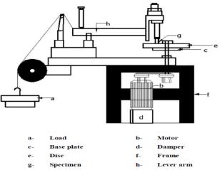
Figure 1. Layout of pin-on-disc apparatus
