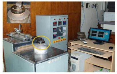
Figure 2 Photograph of pin-on-disc apparatus
