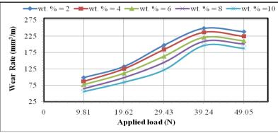
Figure 7. Variation of wear rate with applied load for different wt.% of TiC.
