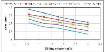
Figure 8. Variation of wear with sliding velocity for different wt.% of TiC.
