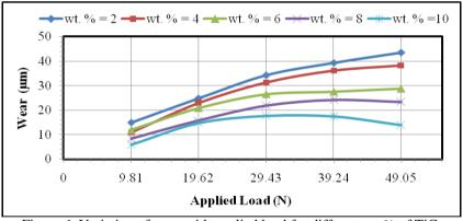
Figure 6. Variation of wear with applied load for different wt.% of TiC.
