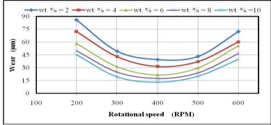
Figure 10. Variation of wear with rotational speed for different wt.% of TiC.
