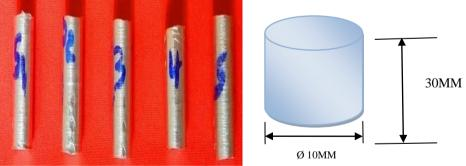
Figure 3 Wear test specimens
