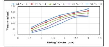
Figure 9. Variation of wear rate with sliding velocity for different wt.% of TiC.
