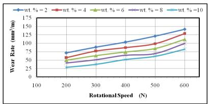
Figure 11. Variation of wear rate with rotational speed for different wt.% of TiC.
