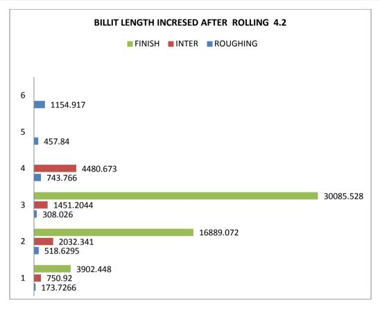
Before rolling the billet size was  $10.1 \times 10.1 \times 150$  cm<sup>3</sup> and when it is passing through roughing inter or finish mill the billet length will increase and the value get on this graph. The actual length is 30085.528cm. before rolling billet weight was 120.116kg and after rolling billet weight 0.586×30085.528×7.85=120.116kg. in this condition the billet volume or density has constant.
