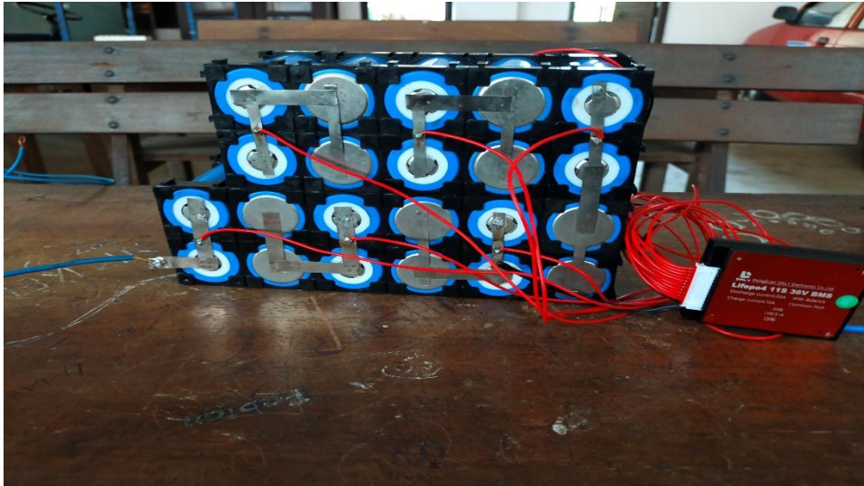
Figure 3 Spot welded battery back with BMS
