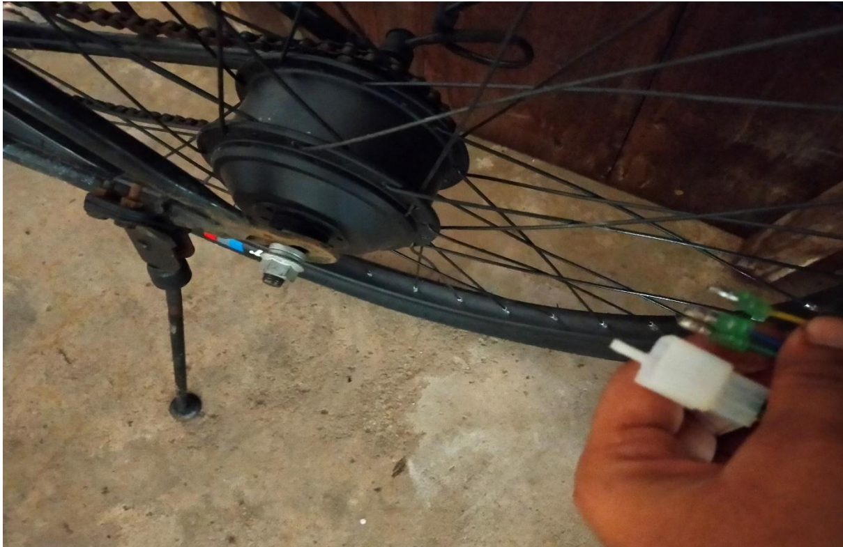
Figure 1: BLDC hub motor of the electric bicycle
