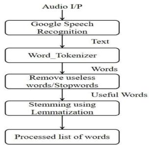
Figure 2 Audio to processed text Dataflow
