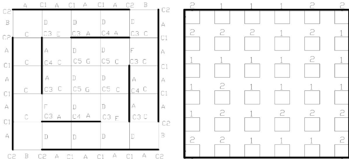
Figure 1.1. (a) Plan view of 9-story buildings, (b) Plan view of isolators for 9-story buildings
