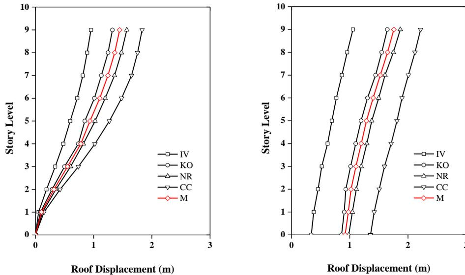
**Figure 1.4. Median (M) and peak displacement distribution in the x directions under selected earthquake for Model A and Model B**
