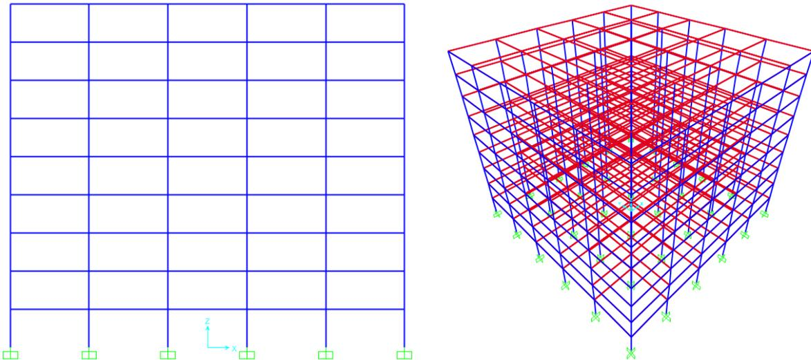
Figure 1.2. Elevation and 3D view of 9-story buildings in SAP 2000
