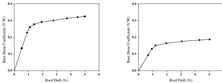
Figure 1.3. Capacity curves for the 9-story conventional building (Model A) and with isolators (Model B)
