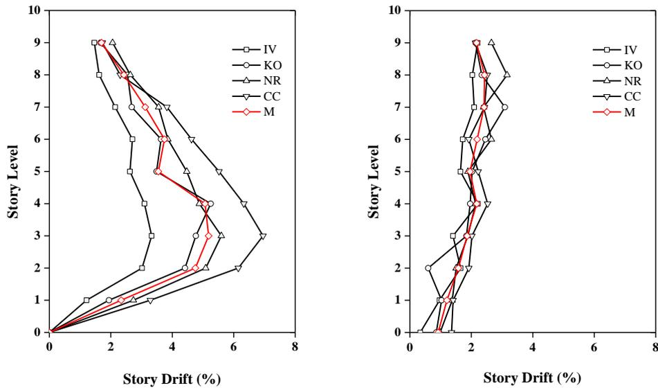
Figure 1.5. Median (M) and story drift distribution in the x directions under selected earthquake for Model A and Model B
