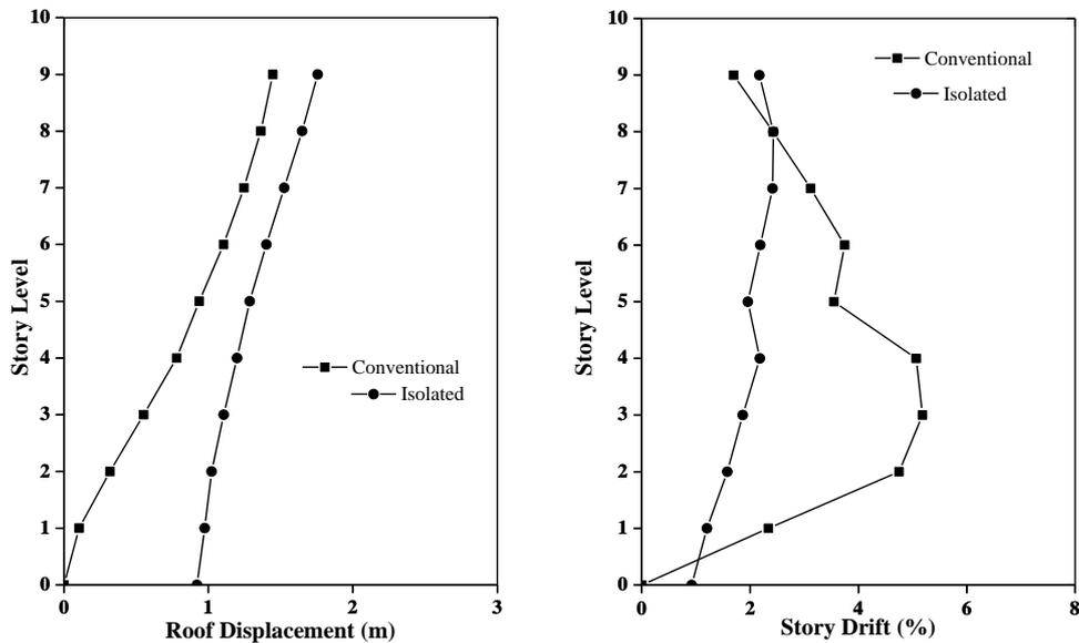
Figure No. 1.6. The median story displacement of 9-story conventional building (Model A) isolated building (Model B) in the four events
