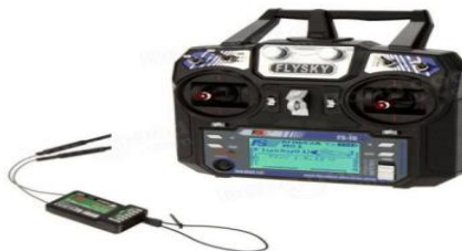
Figure 5 Radio transmitter and receiver
