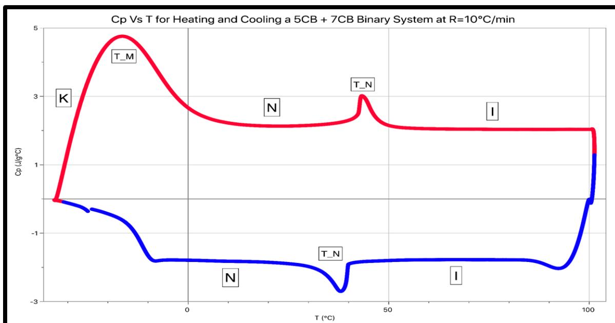
Figure 12.  $C_p$  Vs  $T$  plot for heating (red) and cooling (blue) a 5CB + 7CB BLCS at  $R=10^{\circ}\text{C}/\text{min}$ .
