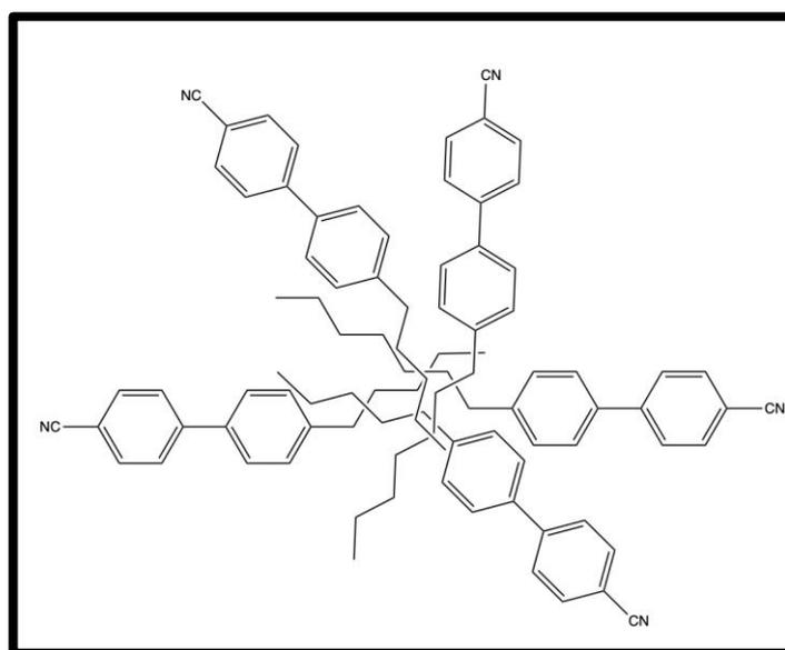
**Figure 31.** Skeletal structure depiction of 5CB and 7CB molecules tail's tangling causing the frozen nematic phenomenon.
