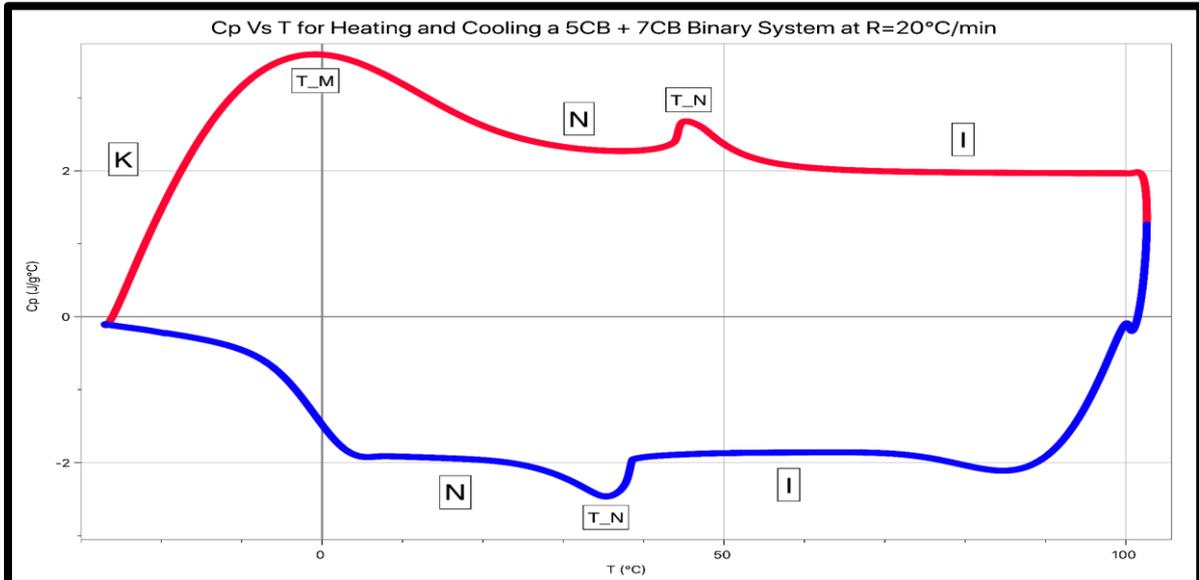
**Figure 13.** Cp Vs T plot for heating (red) and cooling (blue) a 5CB + 7CB BLCS at R=20°C/min.
