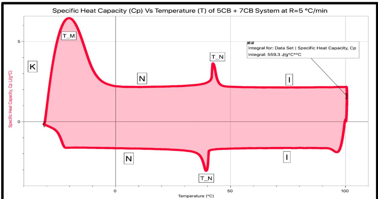
**Figure 8.** Specific Heat Capacity (Cp) Vs T plot for 5CB + 7CB BLCS at R=5°C/min. The shaded area represents the change in internal energy of the mixture during heating and cooling.
