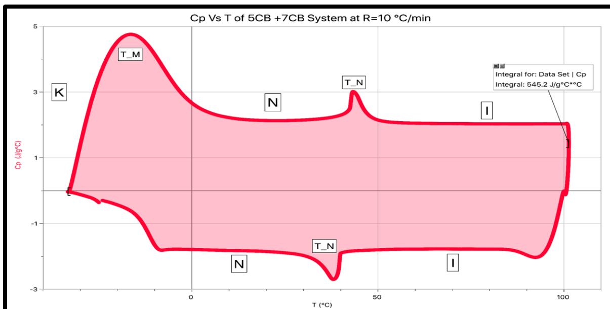
**Figure 9.** Cp Vs T plot for 5CB + 7CB BLCS at R=10°C/min. The shaded area represents the change in internal energy of the mixture during heating and cooling.
