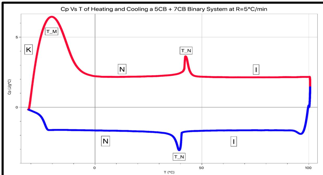
Figure 11.  $C_p$  Vs  $T$  plot for heating (red) and cooling (blue) a 5CB + 7CB BLCS at  $R=5^{\circ}\text{C}/\text{min}$ .
