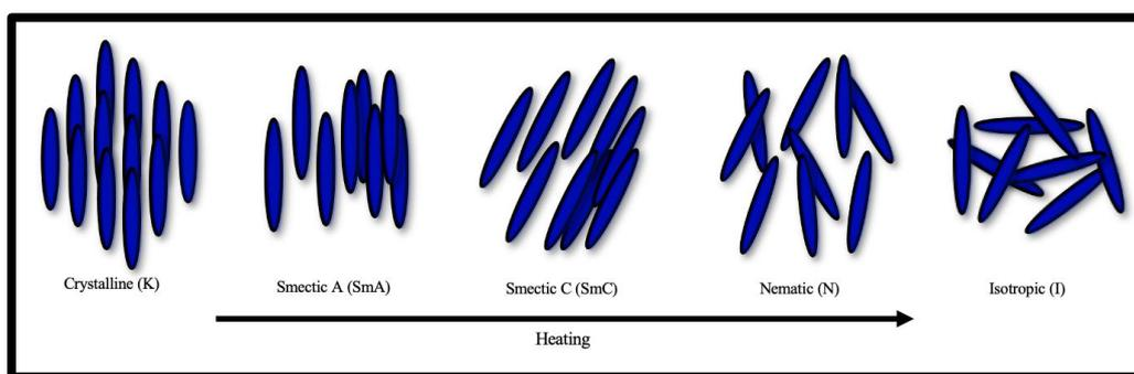
**Figure 1.** Progression of Liquid Crystal Phases during heating.
