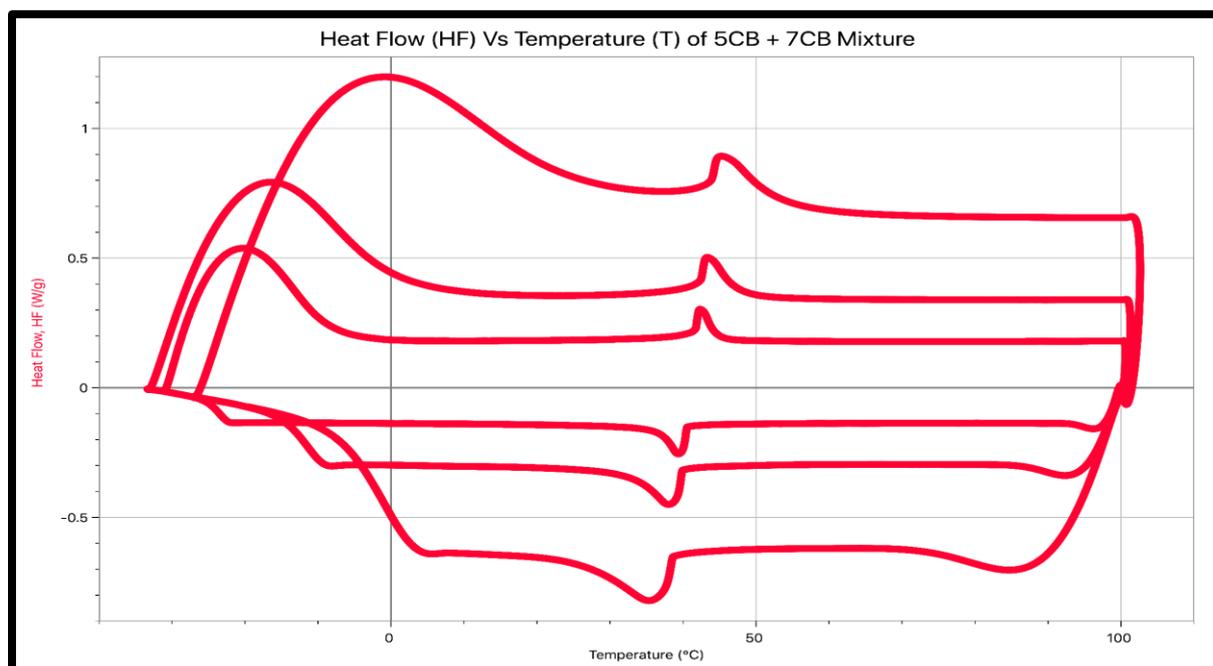
**Figure 4.** Heat Flow Vs Temperature plot for Melting (M) and Nematic (N) phase transitions of 5CB + 7CB BLCS at R= 5,10, and 20°C/min for heating and cooling.
