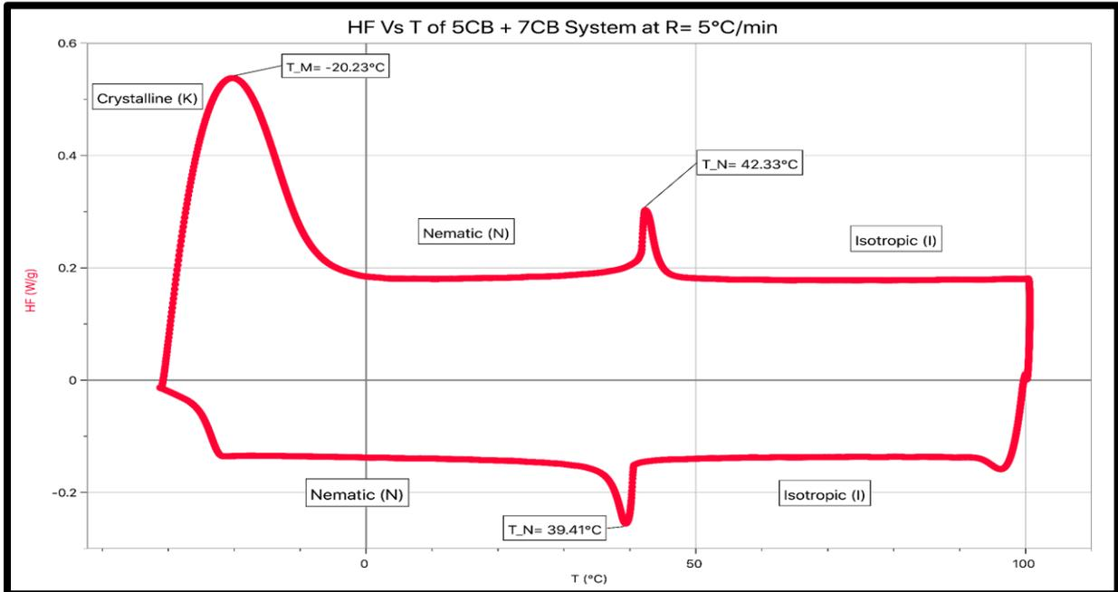
Figure 5. HF Vs T of 5CB + 7CB BLCS for one run of heating and cooling at R=5°C/min.
