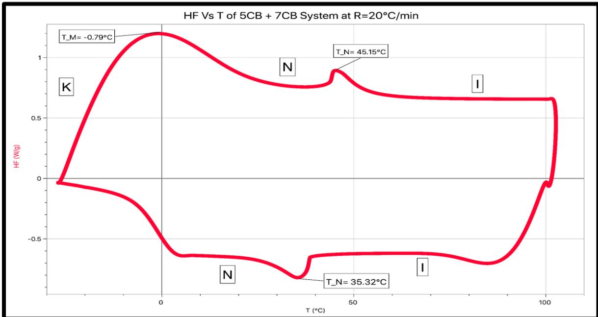
**Figure 7.** HF Vs T of 5CB + 7CB BLCS for one heating and cooling run at R=20°C/min.
