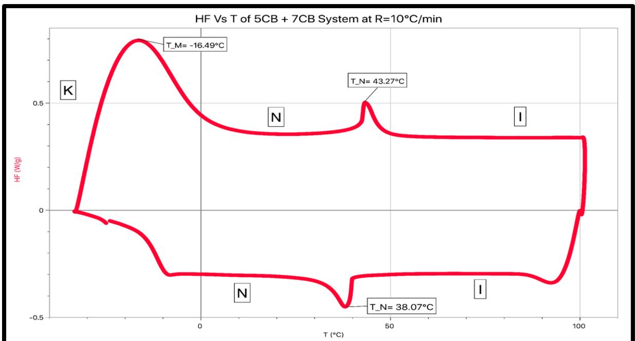
Figure 6. HF Vs T of 5CB + 7CB BLCS for one heating and cooling run at R=10°C/min.
