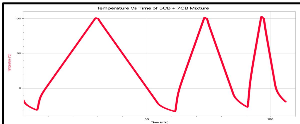
Figure 12. Temperature Vs Time for Three Heating cycles of 5CB + 7CB BLCS at three different rates.
