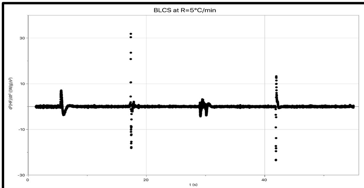
**Figure 4.** Second derivative of heat flow [ $d^2(HF)/dt^2$  Vs t] for heating and cooling a 5CB + 7CB BLCS at  $R=5^\circ\text{C}/\text{min}$ .
