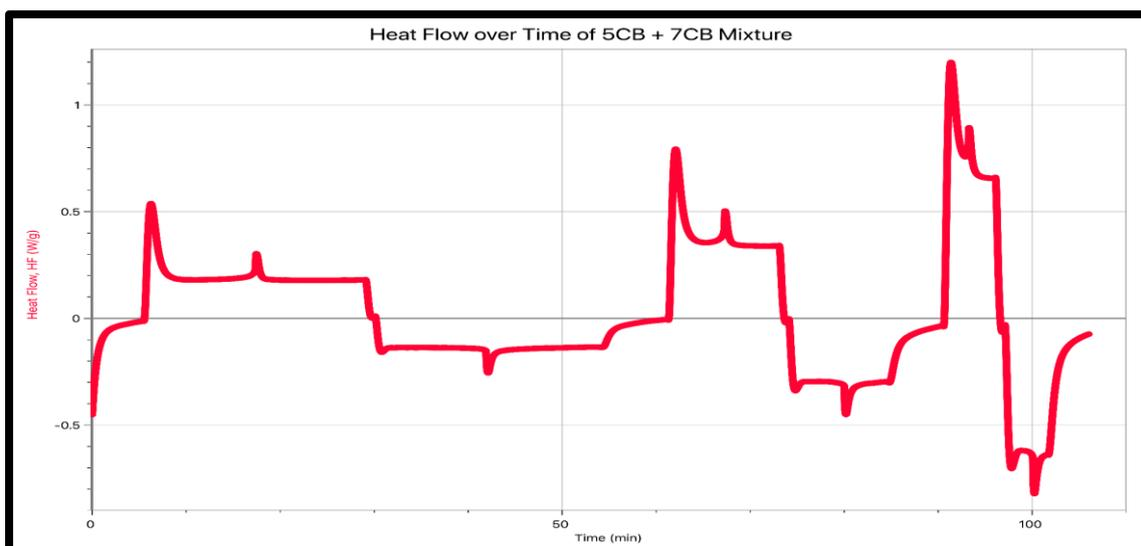
Figure 1. Heat Flow (HF) Vs Time (t) plot for Heating and Cooling a 5CB + 7CB BLCS at rates 5,10, and 20°C/min.
