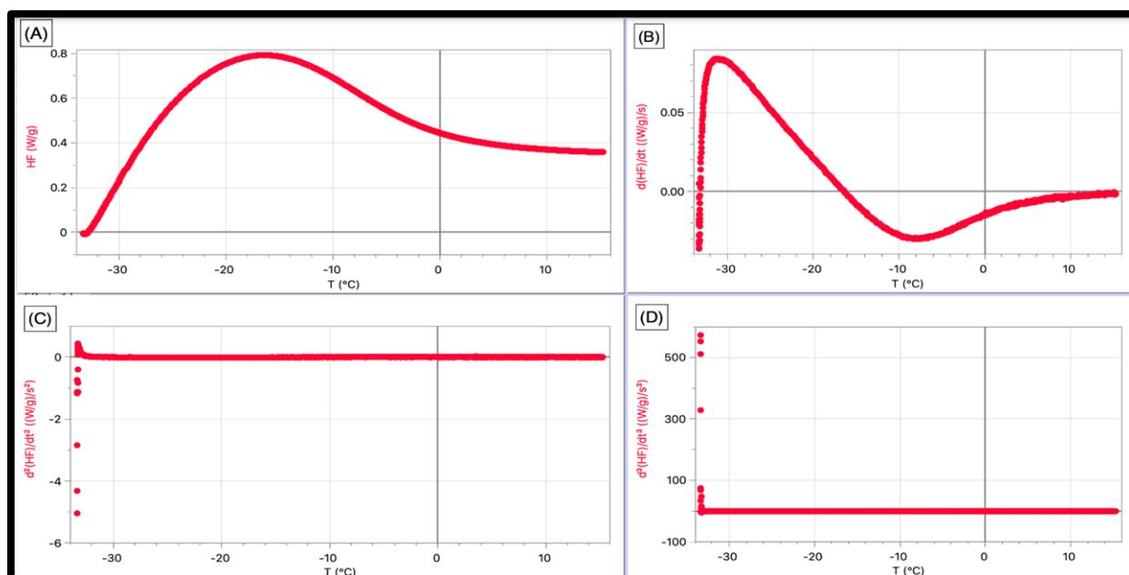
Figure 13. Comparing (a) HF Vs T for Melting transition of 5CB + 7CB BLCS at  $R=10^{\circ}\text{C}/\text{min}$  to its (b) first, (c) second and (d) third derivatives.
