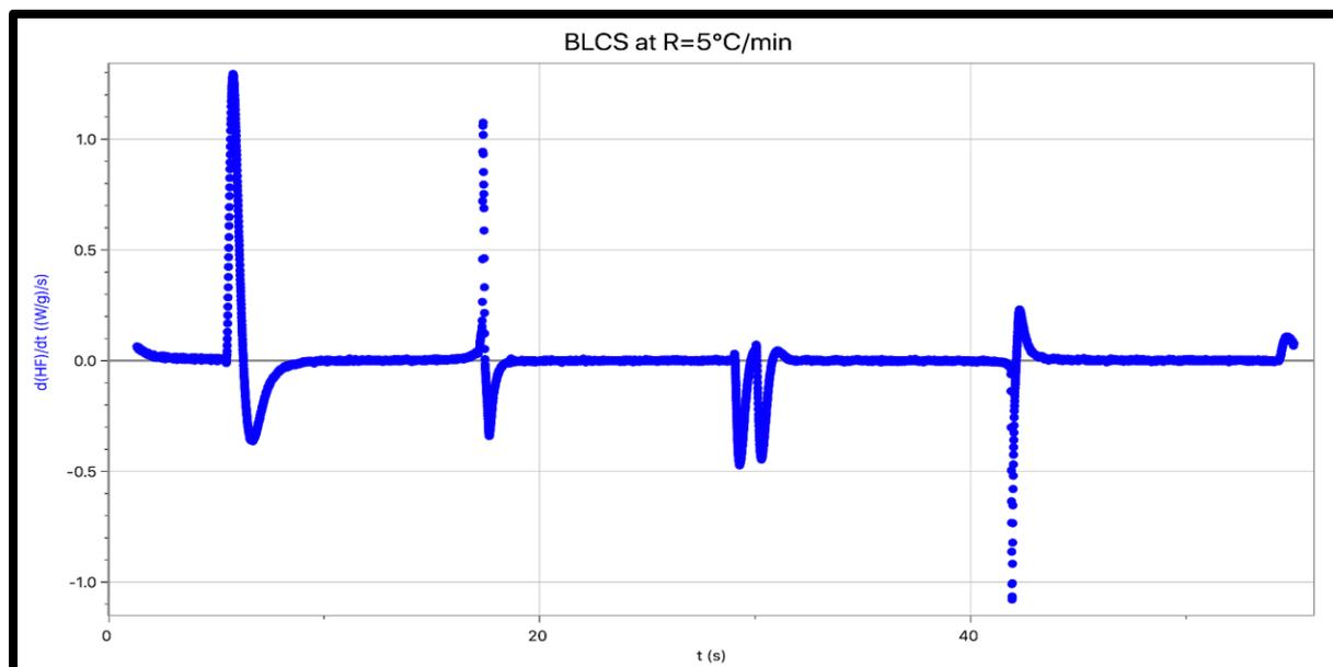
Figure 3. First derivative of heat flow [d(HF)/dt Vs t] for heating and cooling a 5CB + 7CB BLCS at R=5°C/min.
