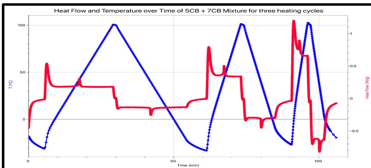
**Figure 11.** HF and T Vs Time of three varied rate heating runs for a 5CB + 7CB mixture.
