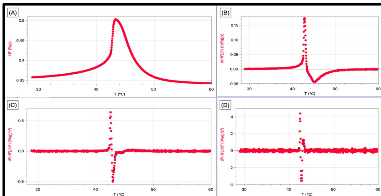
**Figure 14.** Comparing (a) HF Vs T for Heating Nematic transition of 5CB + 7CB BLCS at R=10°C/min to its (b) first, (c) second and (d) third derivatives.
