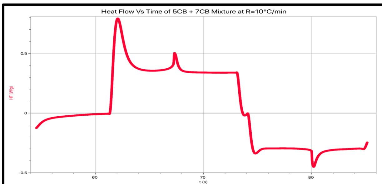
**Figure 5.** HF Vs t plot for Heating and Cooling a 5CB + 7CB BLCS at  $R=10^\circ\text{C}/\text{min}$ .
