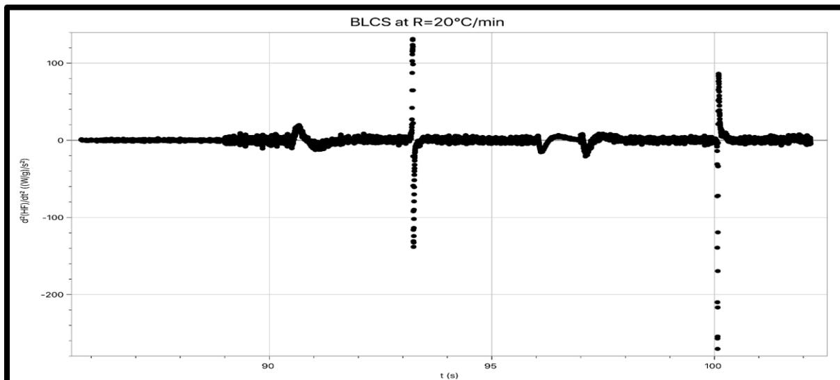
**Figure 10.** Second derivative of heat flow [ $d^2(\text{HF})/dt^2$  Vs  $t$ ] for heating and cooling a 5CB + 7CB BLCS at  $R=20^\circ\text{C}/\text{min}$ .
