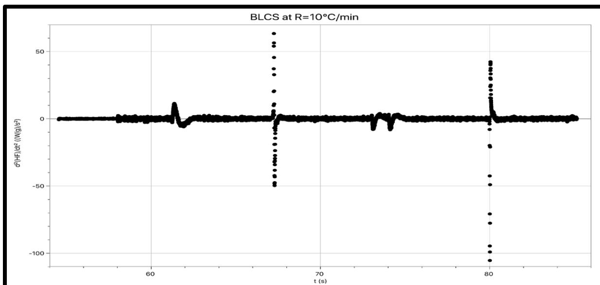
**Figure 7.** Second derivative of heat flow  $[d^2(HF)/dt^2 \text{ Vs } t]$  for heating and cooling a 5CB + 7CB BLCS at  $R=10^\circ\text{C}/\text{min}$ .
