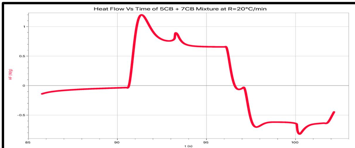
**Figure 8.** HF Vs t plot for Heating and Cooling a 5CB + 7CB BLCS at R=20°C/min.
