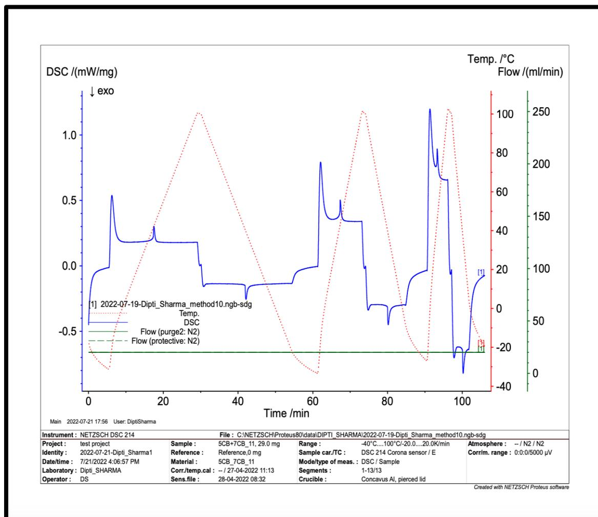
**Figure 17.** Combined all results of BLCS obtained from DSC shown in the form of a pdf file taken from DSC for all three ramp rates 5,10 and 20°C/min as heat flow versus time and temperature plot.
