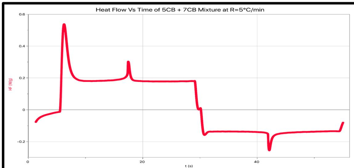
Figure 2. HF Vs t plot for Heating and Cooling a 5CB + 7CB BLCS at R=5°C/min.
