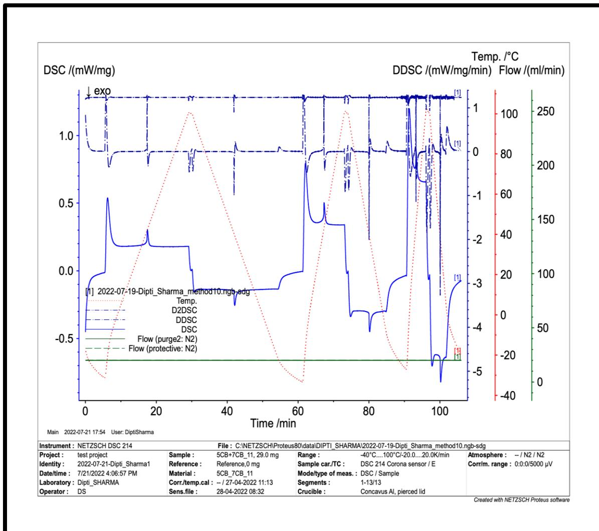
**Figure 18.** Adding twoderivatives of heat flow for the BLCS, all results of BLCS shown in this pdf file are taken from DSC at ramp rates 5,10 and 20°C/min as heat flow versus time.
