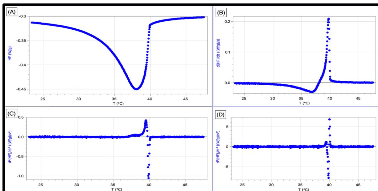
**Figure 15.** Comparing (a) HF Vs T for Cooling Nematic transition of 5CB + 7CB BLCS at R=10°C/min to its (b) first, (c) second and (d) third derivatives.
