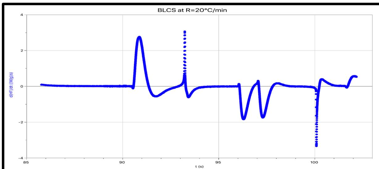
**Figure 9.** First derivative of heat flow [d(HF)/dt Vs t] for heating and cooling a 5CB + 7CB BLCS at R=20°C/min.
