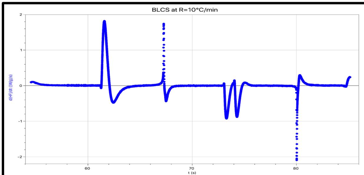
**Figure 6.** First derivative of heat flow  $[d(HF)/dt \text{ Vs } t]$  for heating and cooling a 5CB + 7CB BLCS at  $R=10^\circ\text{C}/\text{min}$ .
