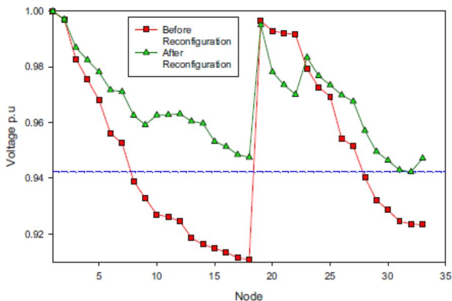
Fig. 4. Voltage Profile of IEEE 69 Bus system Before & After Reconfiguration by MPSO.
