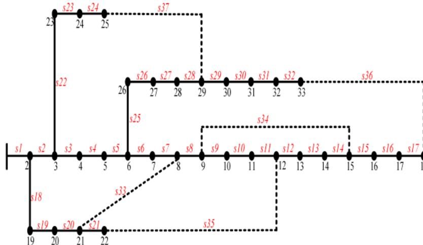
Fig. 3. Single Line Diagram of IEEE-33 Bus System
