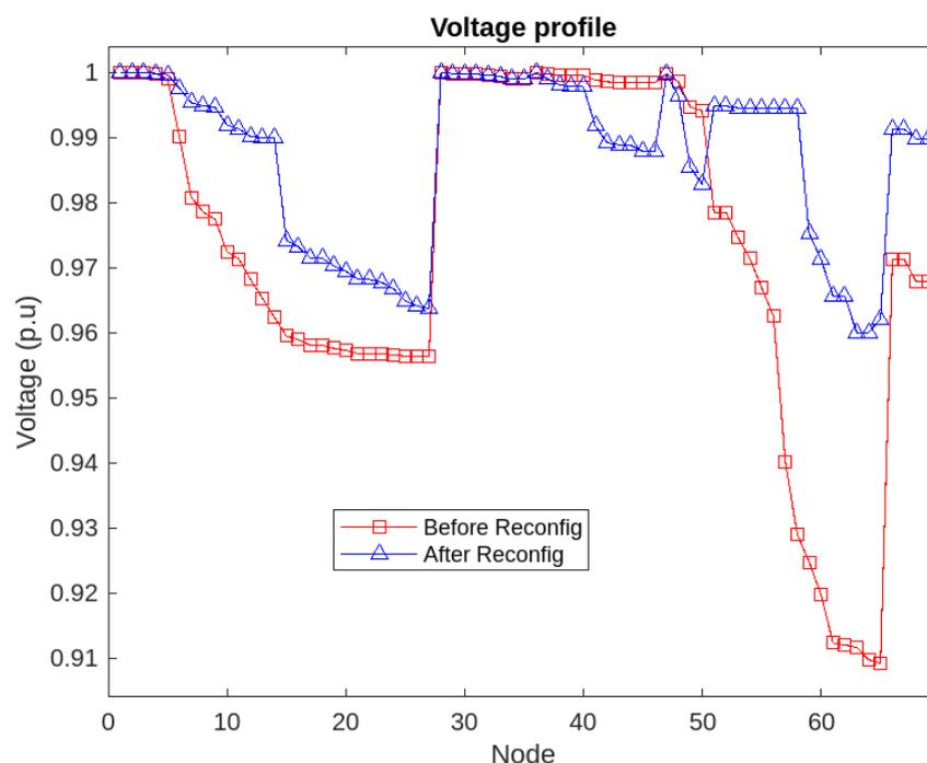
**Fig. 6. Voltage Profile of IEEE 69 Bus system Before & After Reconfiguration by MPSO**
