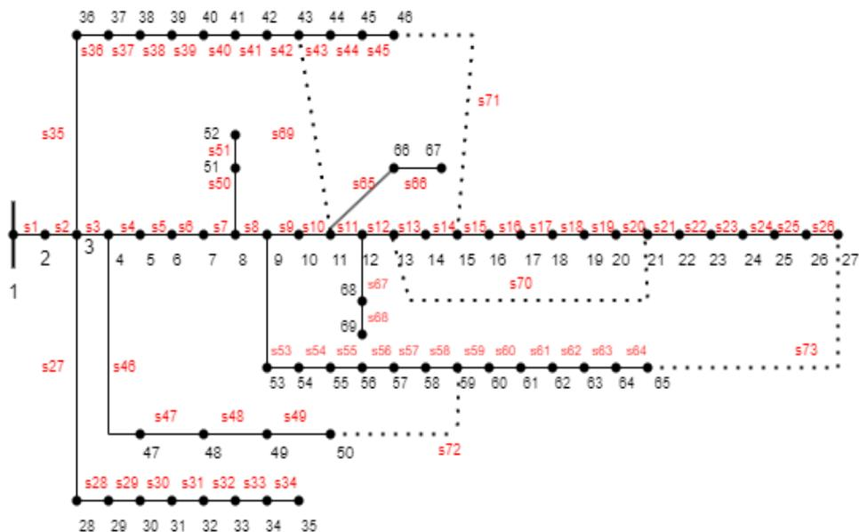
Fig. 5. Single Line Diagram of IEEE-69 Bus System
