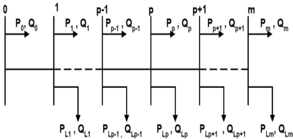
Fig. 1. Single Line Diagram of Main Feeder
