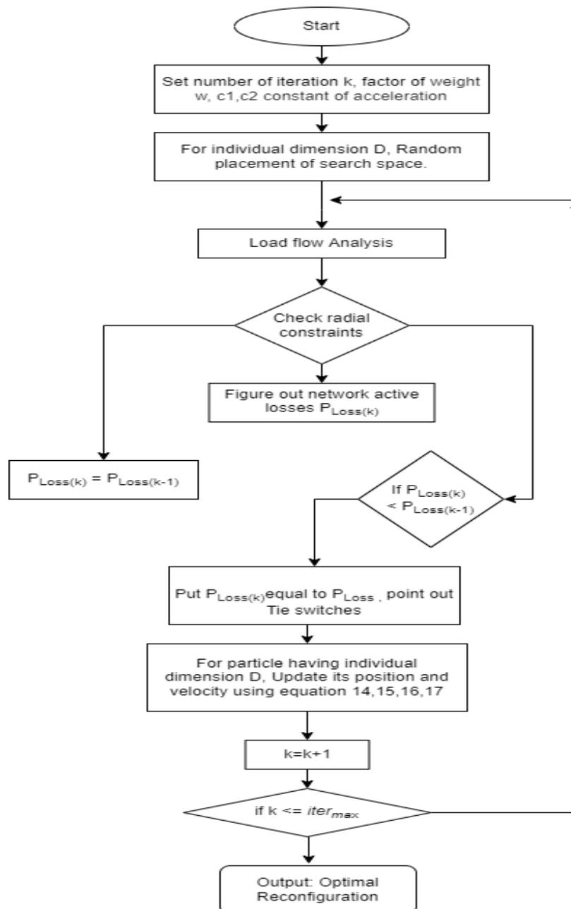
Fig. 2. Flowchart of MPSO method
