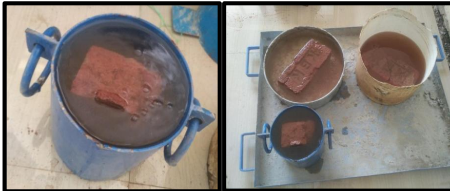
Figure 3.2: Water Absorption of Bricks Source: Shivajirao S Jondhle Polytechnic, Asangaon
