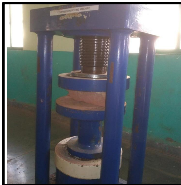
Figure 3.3: Compressive Strength Test Machine Source: Shivajirao S Jondhle Polytechnic, Asangaon
