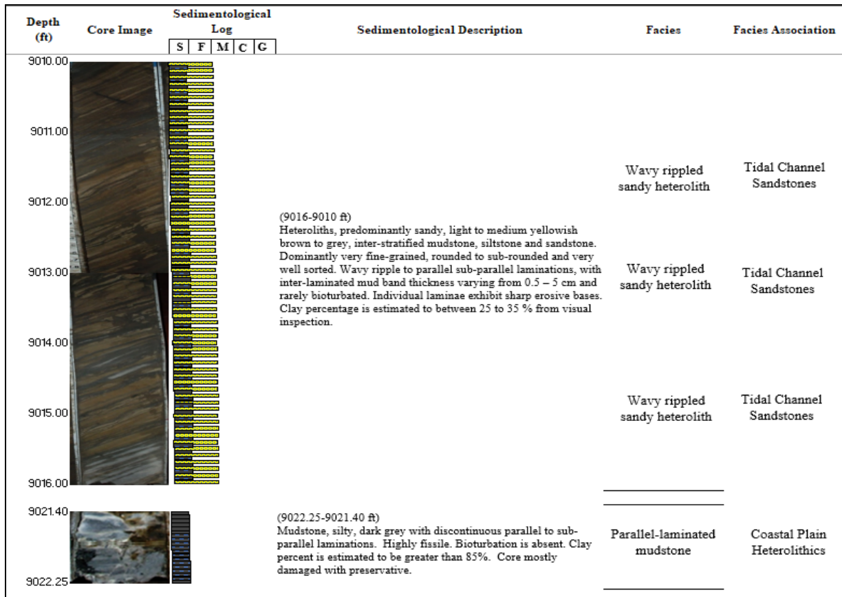
Figure 8.4: Results of Sedimentological Analysis (Litholog) and Facies description from a depth range of 9022.25 - 9010ft
