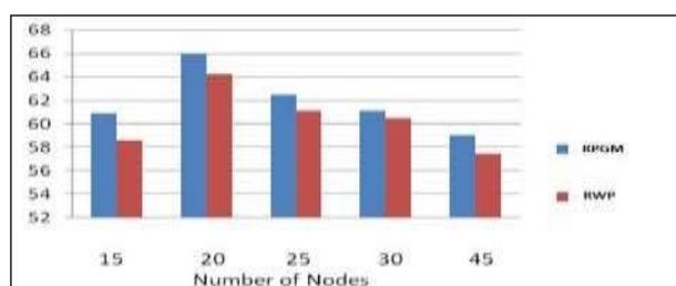
Figure 4. Routing Overhead vs. Number of Nodes
